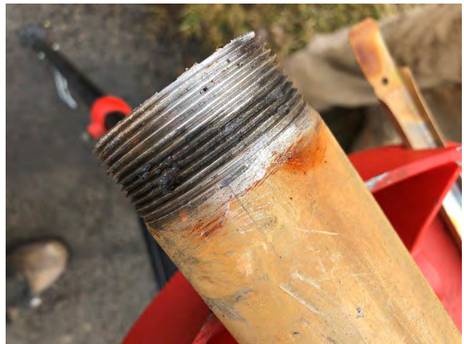
View of recovery well RW-1 pump riser damaged threads.
