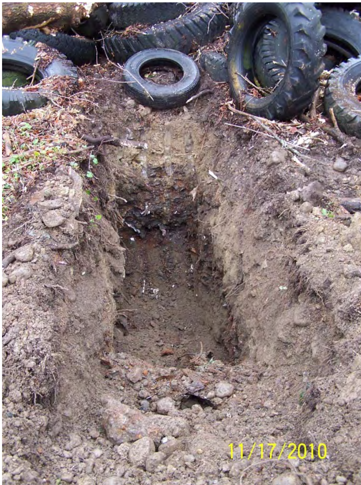
Photo 7605. Solid waste layer (approximately 2 ft thick) in TP-5, looking toward slope.
