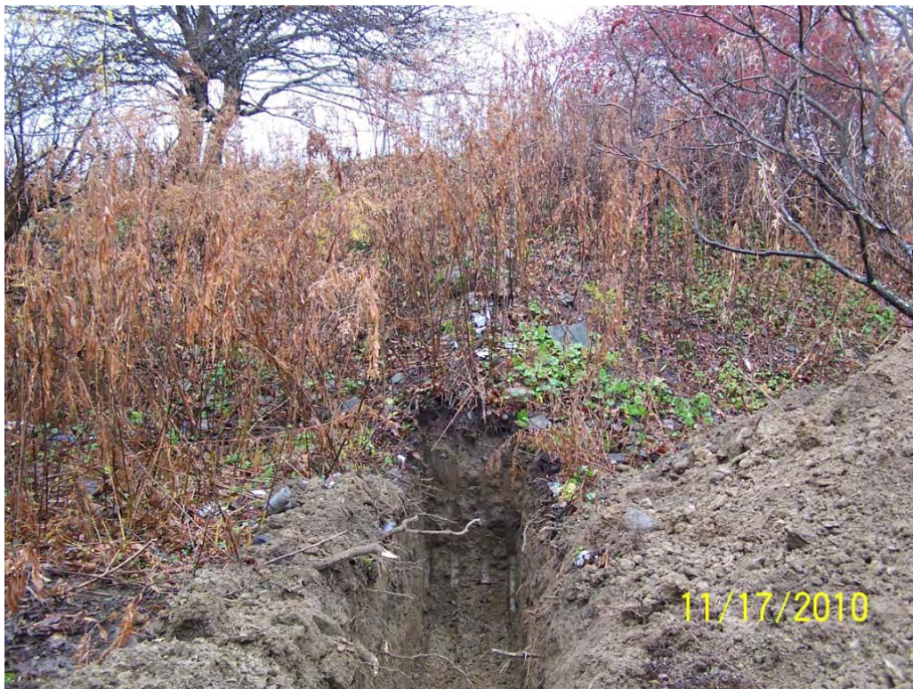
Photo 7611. No solid waste layer in TP-6, looking toward slope.
