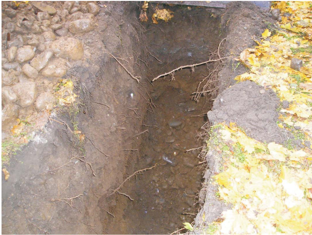
Photo #7: Test trench TP-01 excavated to approximately 7.5 feet below ground surface, looking southeast. Thin ash layer visible at approximately 1.5 feet below ground surface.
