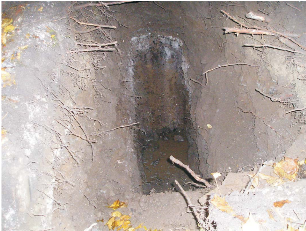
Photo #9: Test trench TP-03 excavated to approximately 10.5 feet below ground surface, looking west. Note ash layer at approximately 6.0 feet below ground surface. Perched water encountered at 10.5 feet below ground surface.
