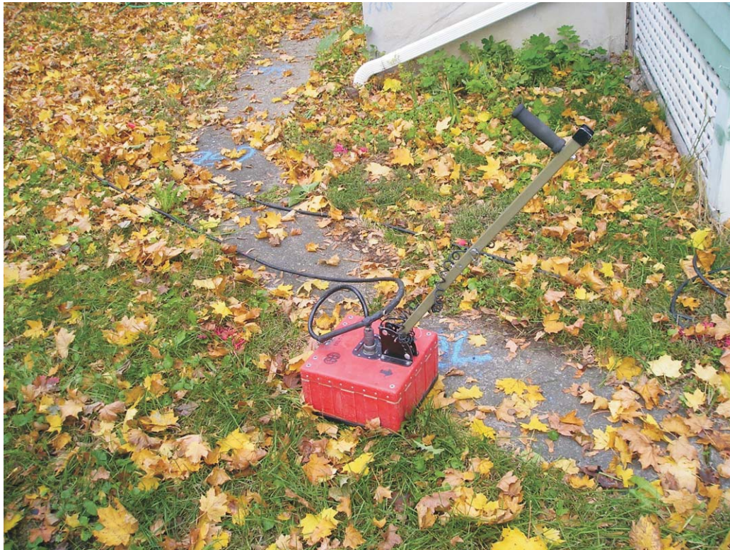
Photo #6: Close-up of GPR apparatus.
