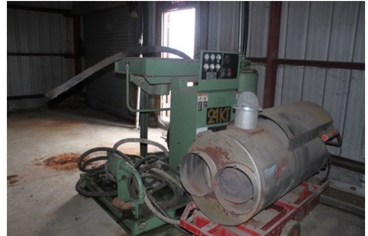
Photo 26 Frost-Fighter forced-air heating system portable heater.
