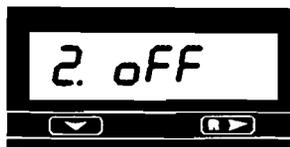
**Mode #2: Totalizer Decimal Point:** Sets the decimal point on the totalizer display from no decimal (off) to 0.00000
