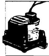
Set any point within the adjustable range—an increase or decrease in pressure will open or close the circuit. Switches have NEMA 4 watertight enclosure and tamper-resistant, external adjustment screws. Pressure (vacuum) connection is 1/4" FPT. Electrical connection is 1/2" NPS conduit.
