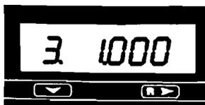
**Mode #3: Rate Scale Factor Decimal Point:** Sets the decimal point in the Rate Scale Factor number from no decimal to 0.000.
