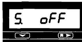
**Mode #5: Rate Decimal Point:** Sets the decimal point on the Rate of Flow display from no decimal (off) to 0.000. You can also program the display to have a dead zero (----0), for a 5 digit display with the least significant digit always being "0".
