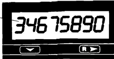
**Rate Display:** Indicates the rate value, which is equal to the input frequency multiplied by the Rate Scaler Value in Program Mode #3. (If no pulses are received for 2 seconds, the rate value goes to zero.)
