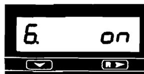
**Mode #6: Front Panel Reset Enable:** When programmed "on" the
