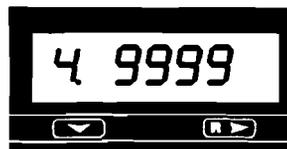
**Mode #4: Rate Scale Factor:** Multiplies the input pulses by this number, which can be programmed in conjunction with the Rate Decimal Point for a number from 0.001 to 9999.
