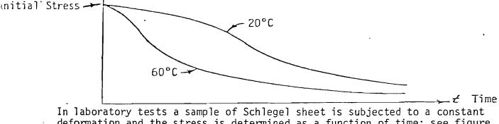
deformation and the stress is determined as a function of time; see figure below.
