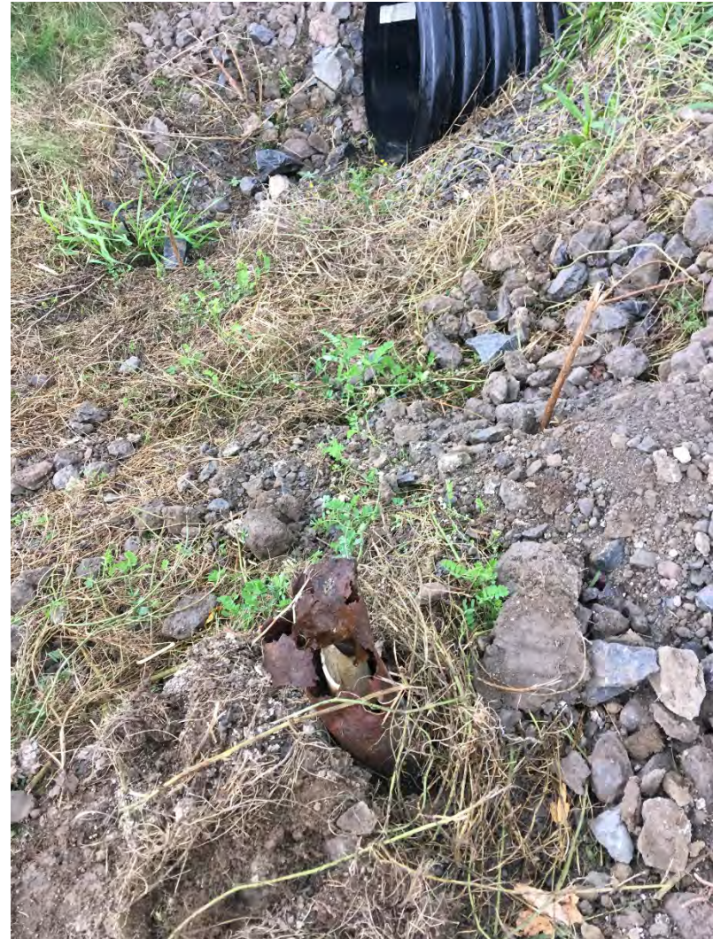
24. View of damaged groundwater monitoring well DW-103 in vicinity of recent construction activities completed by others.
