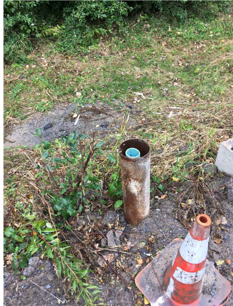
8. View of Inclinator 2 (interior pipe used as Site benchmark). Cover was found to be off and was loosely replaced.
