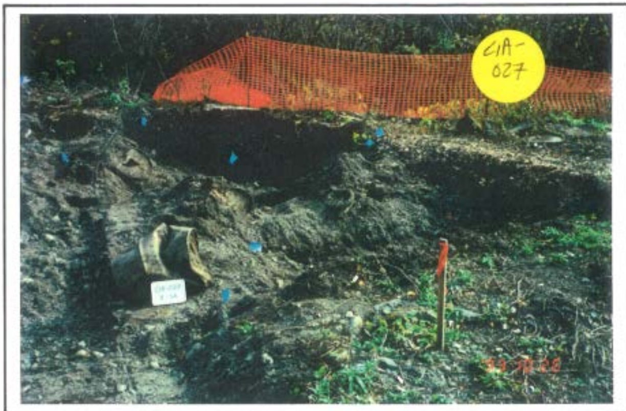
Photograph 8 - Test Pit CIA-027 - Blue Flags Locate Individual Drums Partially Uncovered
