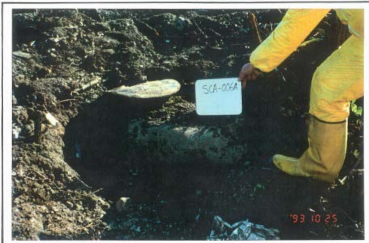
Photograph 5 - Test Pit SCA-006 A - Partially Uncovered Drum
