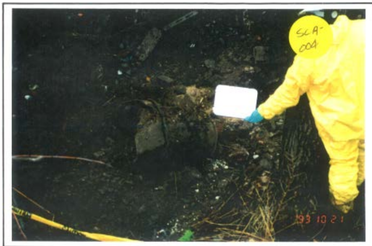
Photograph 4 - Test Pit SCA-004 - Uncovered Drum Showing Deteriorated Condition
