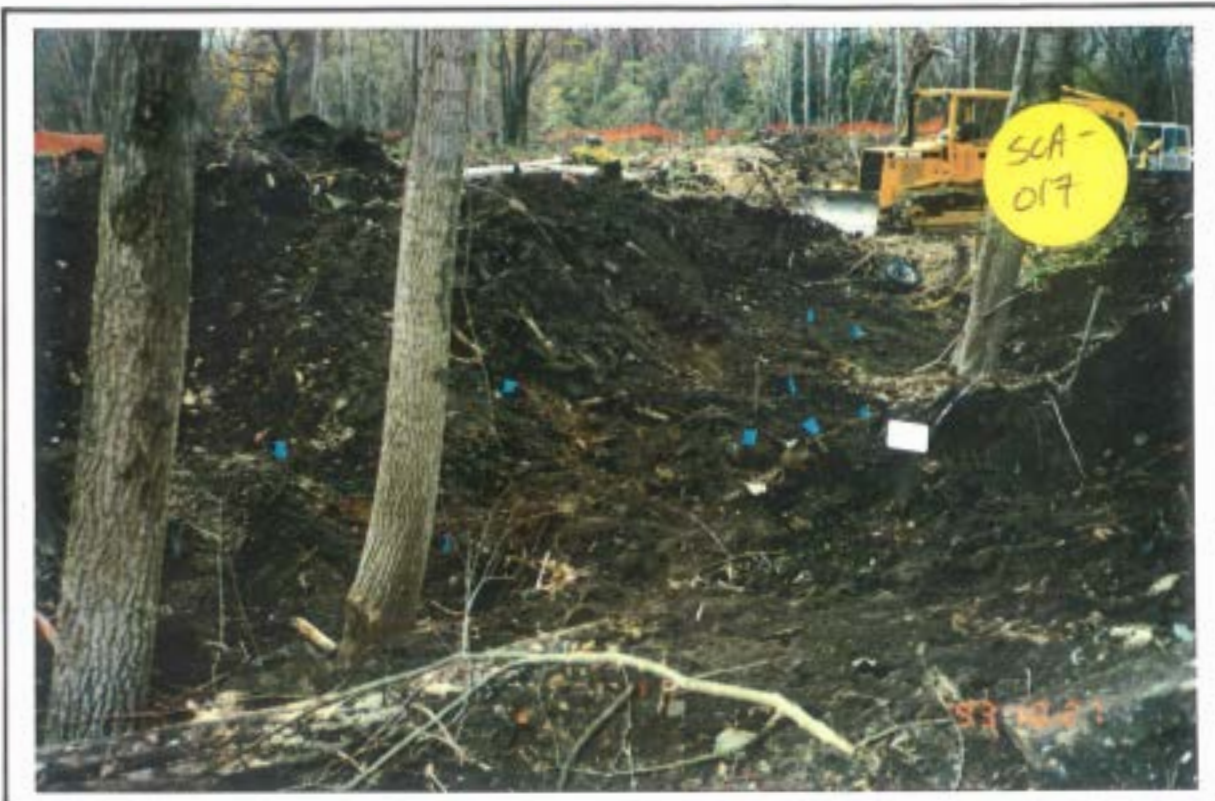
Photograph 6 - Test Pit SCA-017 - Blue Flags Locate Individual Drums Partially Uncovered
