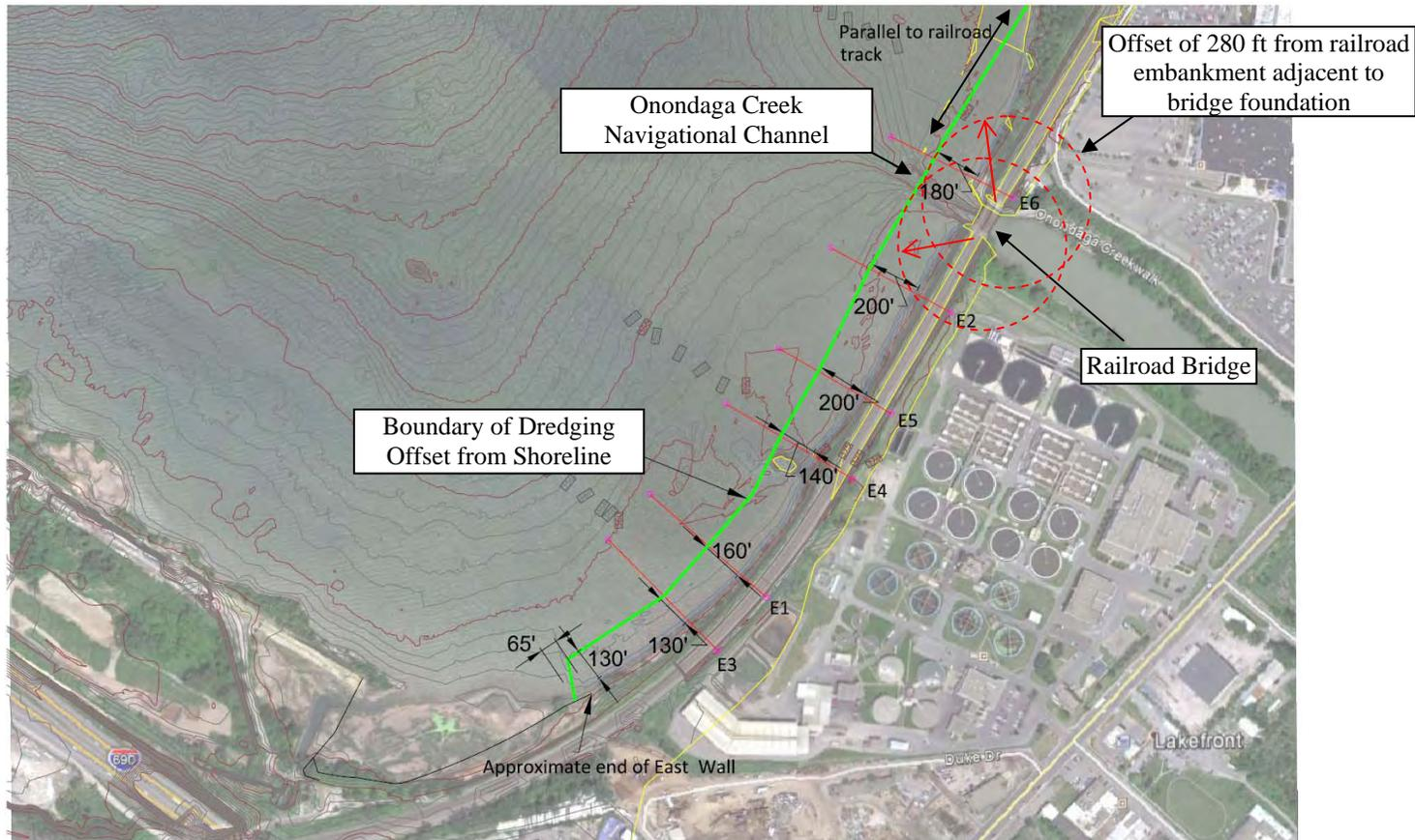
Figure 10. Minimum Required Dredge Offset Distance and Recommended Boundary of No-Dredging Area
