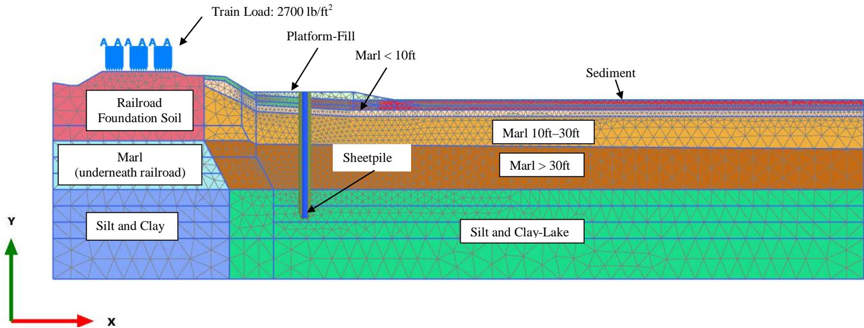
Figure 8. Geometry and Subsurface Layers Used in Finite Element Analysis of Cross Section E5 where sheetpile is 30 ft away from the shoreline
