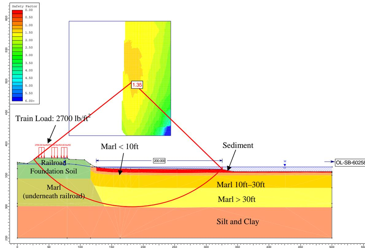
Figure 8. Geometry and Slope Stability Analysis Results of Cross Section E5 (with Offset Distance of 200 ft from the Shoreline)
