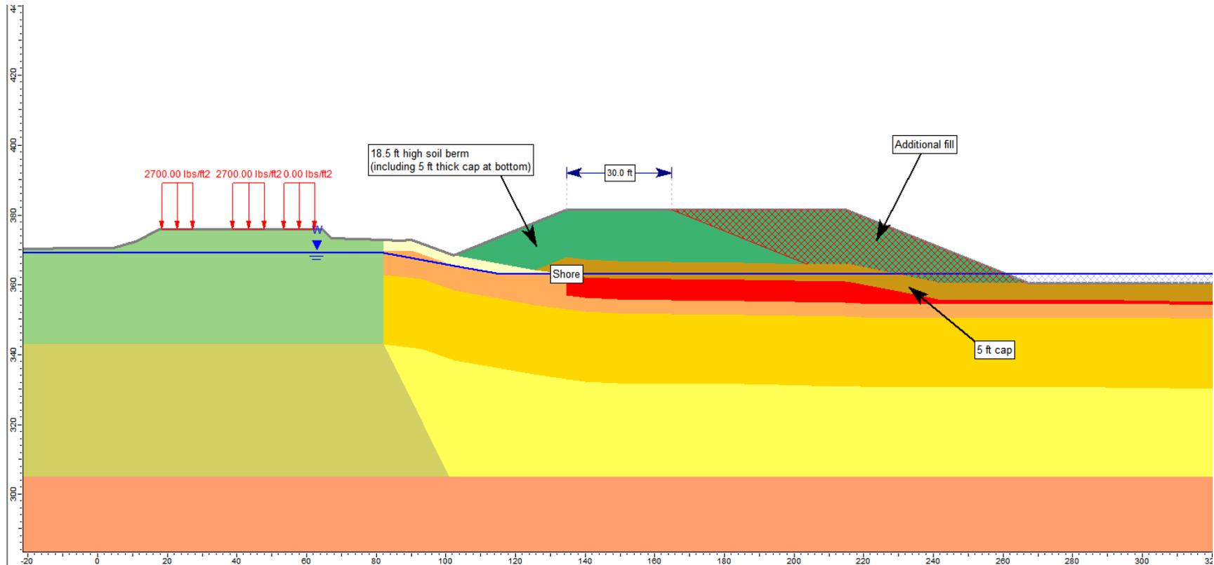
Figure 1D. Stage 4 of Surcharge Placement Sequence: Placement of Additional Fill in front of Soil Berm at Year 2
