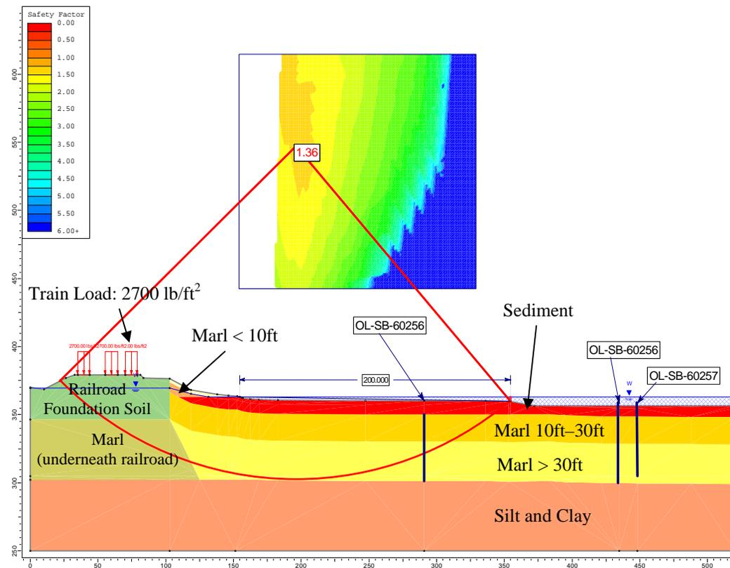
Figure 5. Geometry and Slope Stability Analysis Results of Cross Section E2 (with Offset Distance of 200 ft from the Shoreline)
