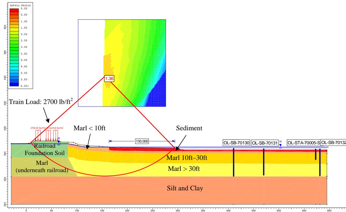
Figure 6. Geometry and Slope Stability Analysis Results of Cross Section E3 (with Offset Distance of 130 ft from the Shoreline)
