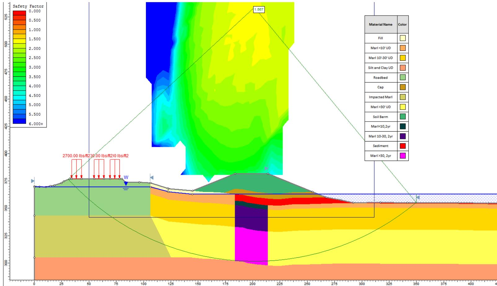
Figure 6. Slope Stability Analysis Results – 18.5-ft Surcharge, Section E4, Stage 2
