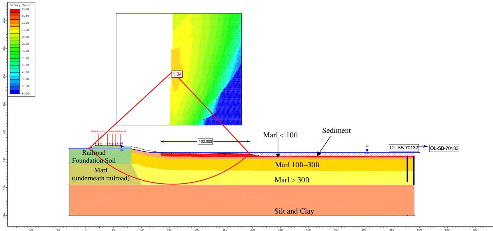
Figure 4. Geometry and Slope Stability Analysis Results of Cross Section E1 (with Offset Distance of 160 ft from the Shoreline)
