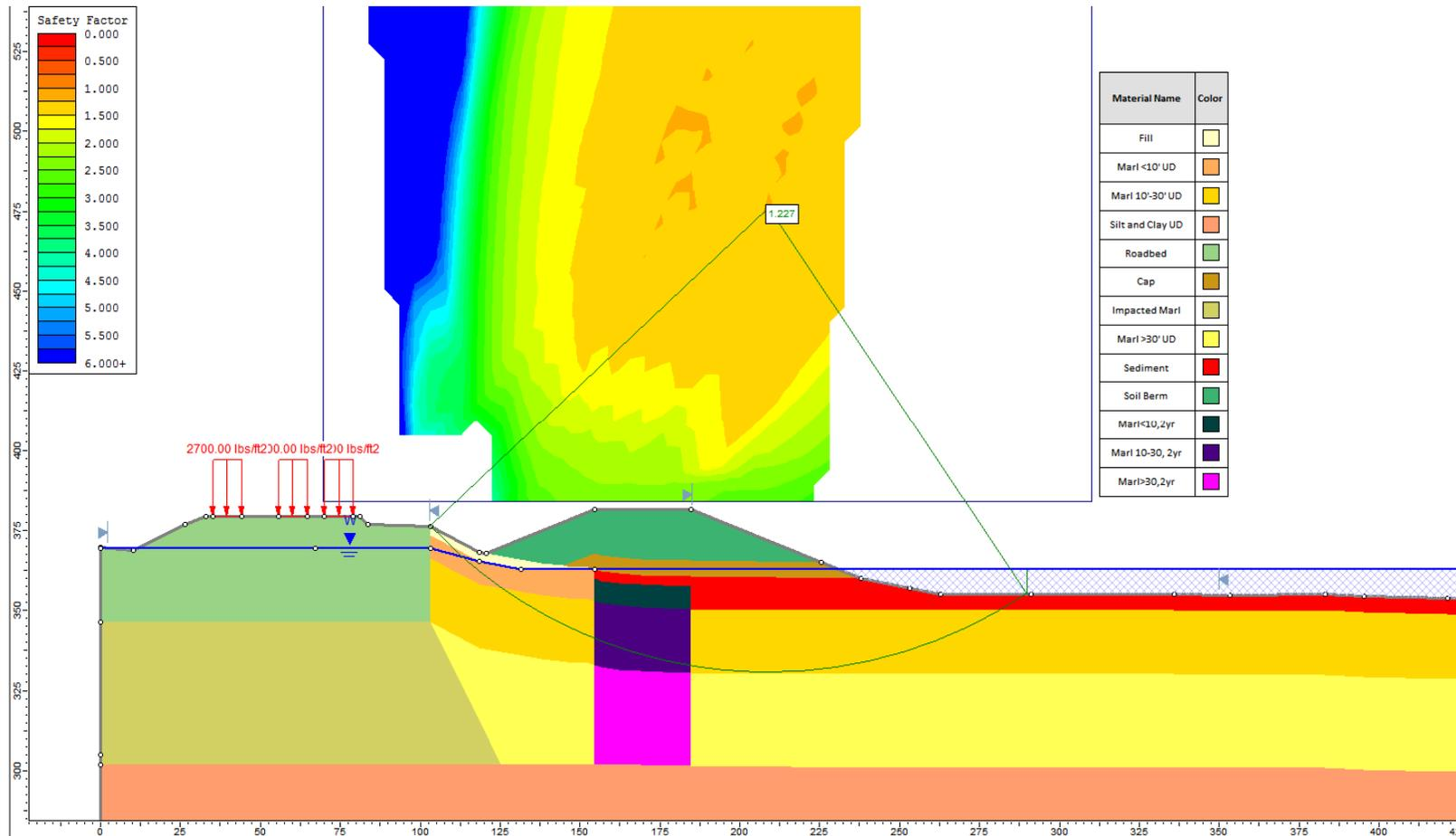
Figure 4. Slope Stability Analysis Results – 18.5-ft Surcharge, Section E2, Stage 2
