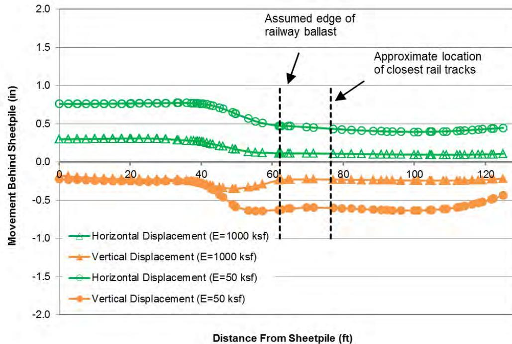
Figure 11. Calculated Vertical and Horizontal Deformation Profiles at Cross Section E5 where sheetpile is located 30 ft away from the shoreline (Railroad Foundation Soil Modulus,  $E = 50$  and  $1000$  ksf)
