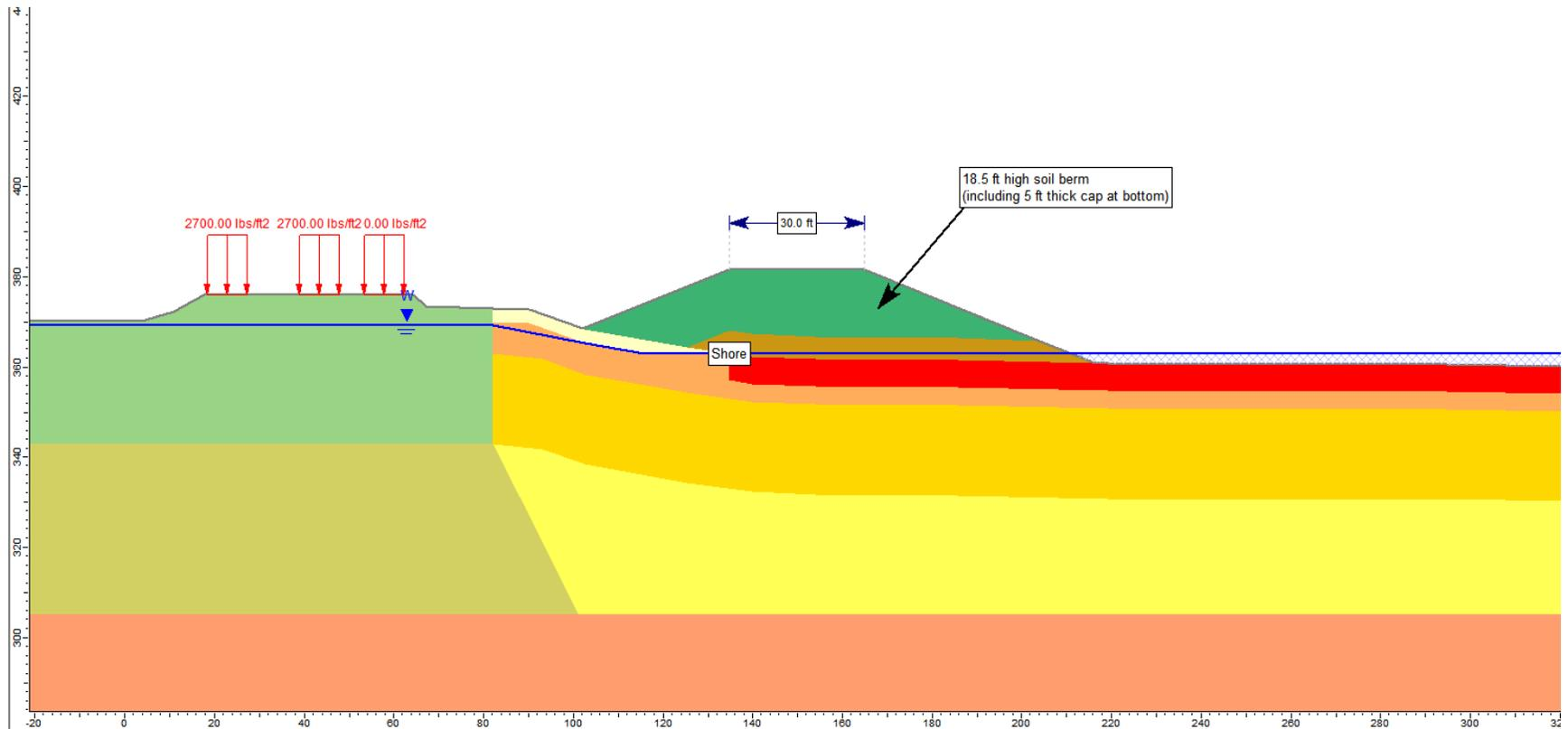
Figure 1A. Stage 1 of Surcharge Placement Sequence: Construction of Soil Berm at Year 0
