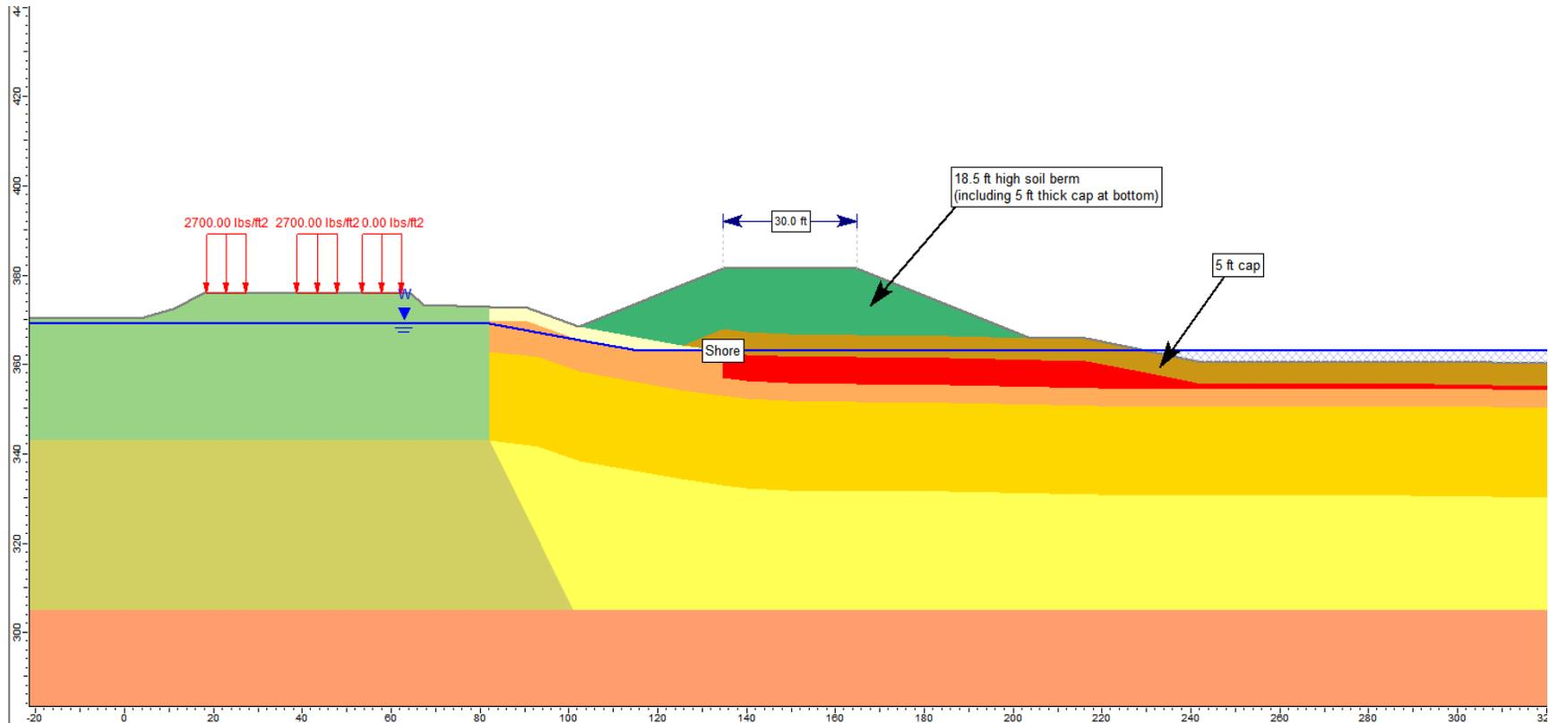
Figure 1C. Stage 3 of Surcharge Placement Sequence: Construction of Cap in front of Soil Berm at Year 2
