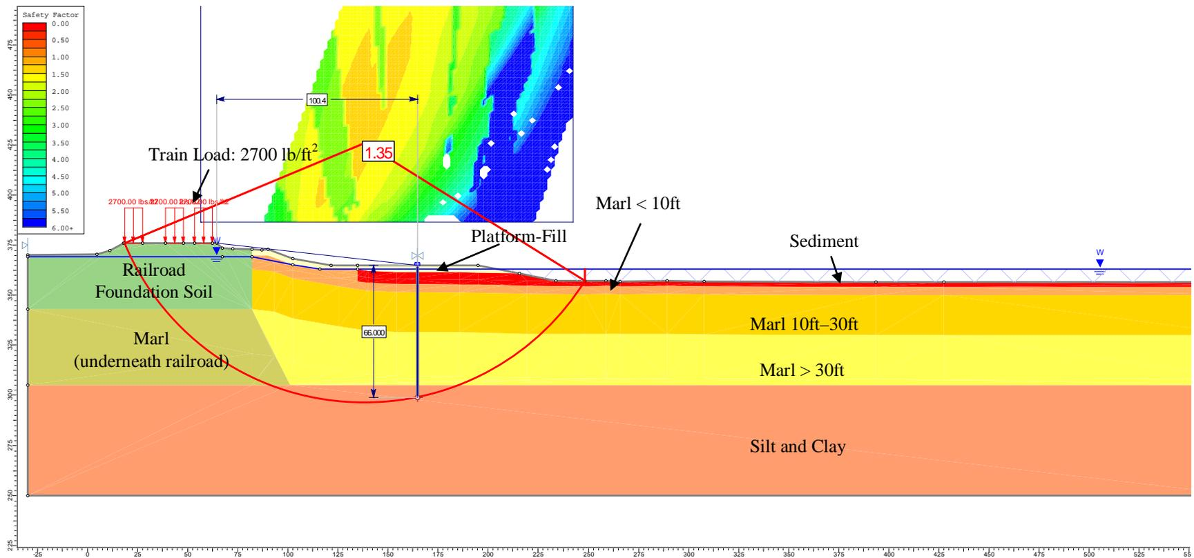
Figure 2. Geometry and Slope Stability Analysis Results of Cross Section E1 where sheetpile is 30 ft away from the shoreline
