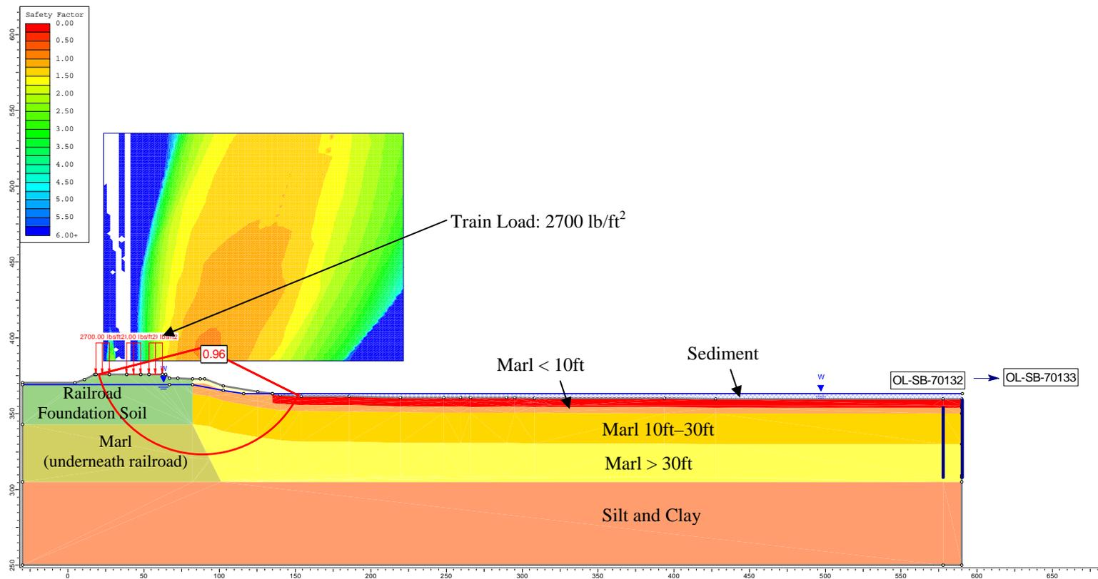
Figure 3. Slope Stability Analysis Results of Cross Section E1 for the Existing Condition
