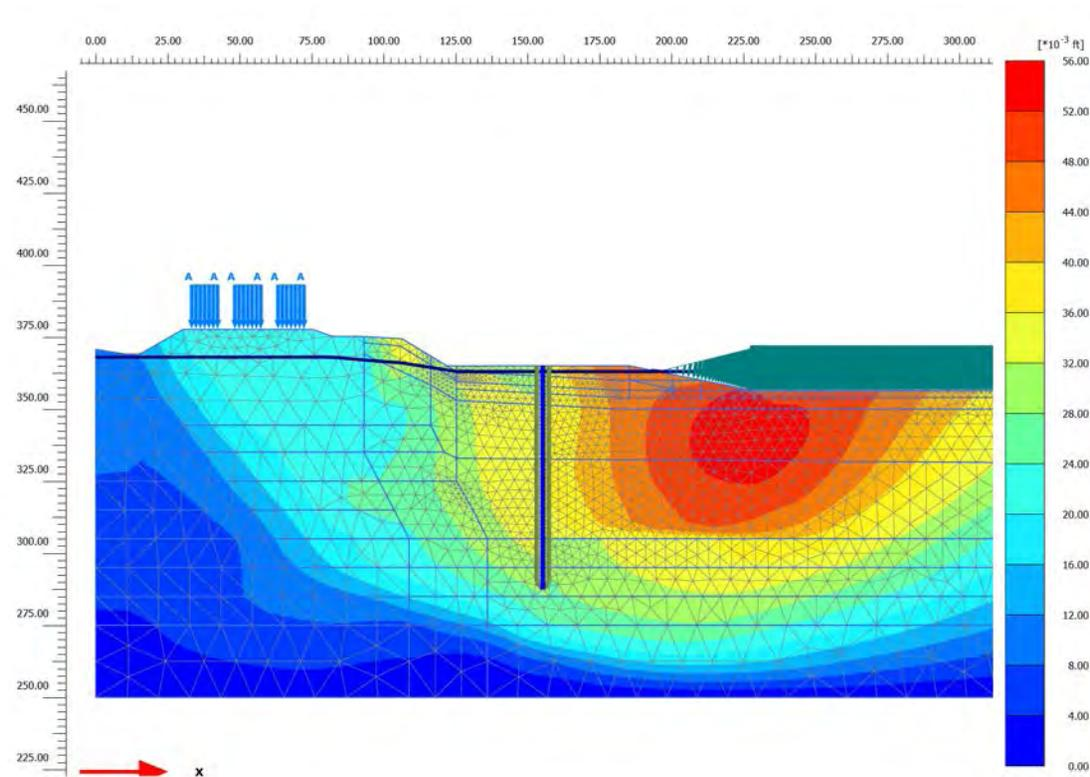
Figure 9. Calculated Deformation Contours after Dredging in front of Sheetpile at Cross Section E5
