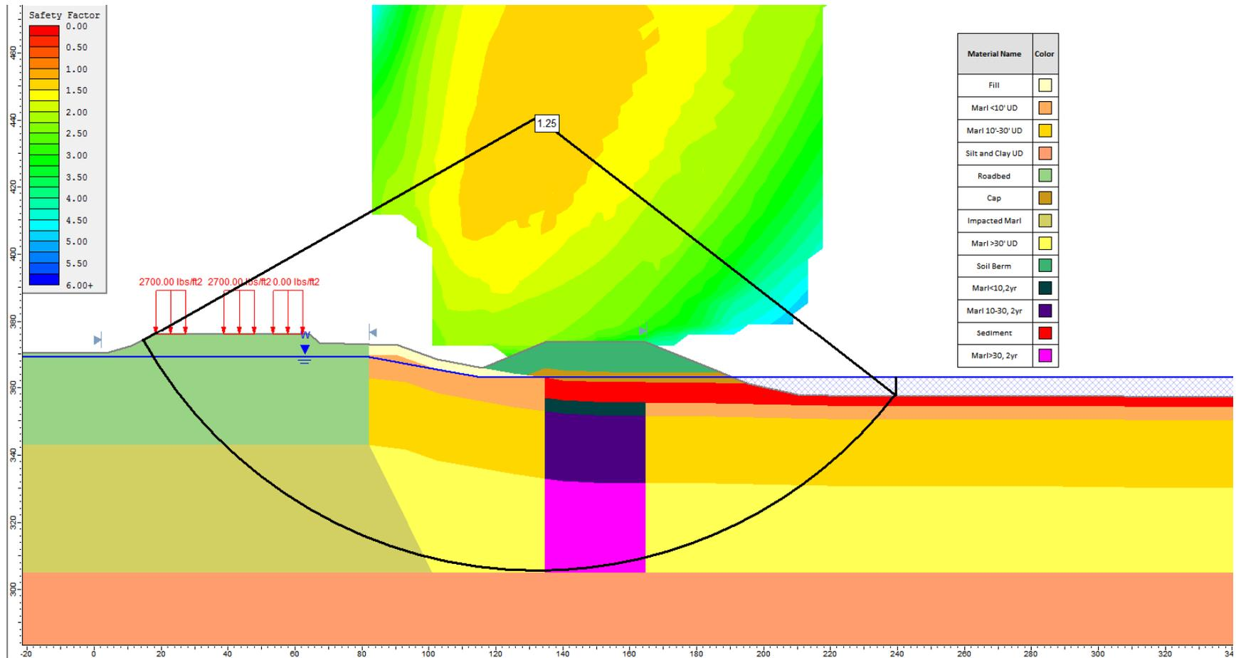
Figure 9. Slope Stability Analysis Results – 10.5-ft Surcharge, Section E1, Stage 2
