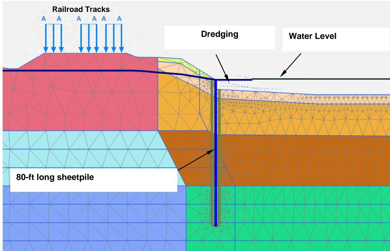
**Finite Element Mesh (Cross Section)**
