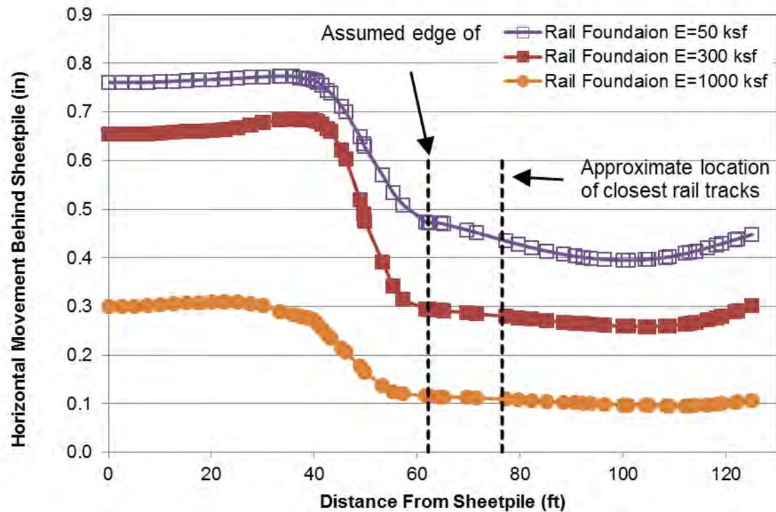
Figure 10. Sensitivity of Calculated Horizontal Deformation to Modulus of Railroad Foundation at Cross Section E5 where sheetpile is located 30 ft away from the shoreline (Railroad Foundation Soil Modulus, E = 50, 300, and 1000 ksf)
