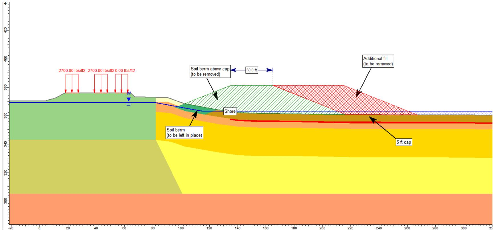
Figure 1E. Stage 5 of Surcharge Placement Sequence: Removal of Soil Berm at End of Year 5
