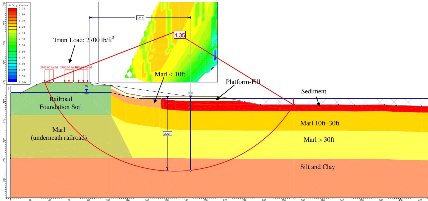
Figure 3. Geometry and Slope Stability Analysis Results of Cross Section E2 where sheetpile is 30 ft away from the shoreline
