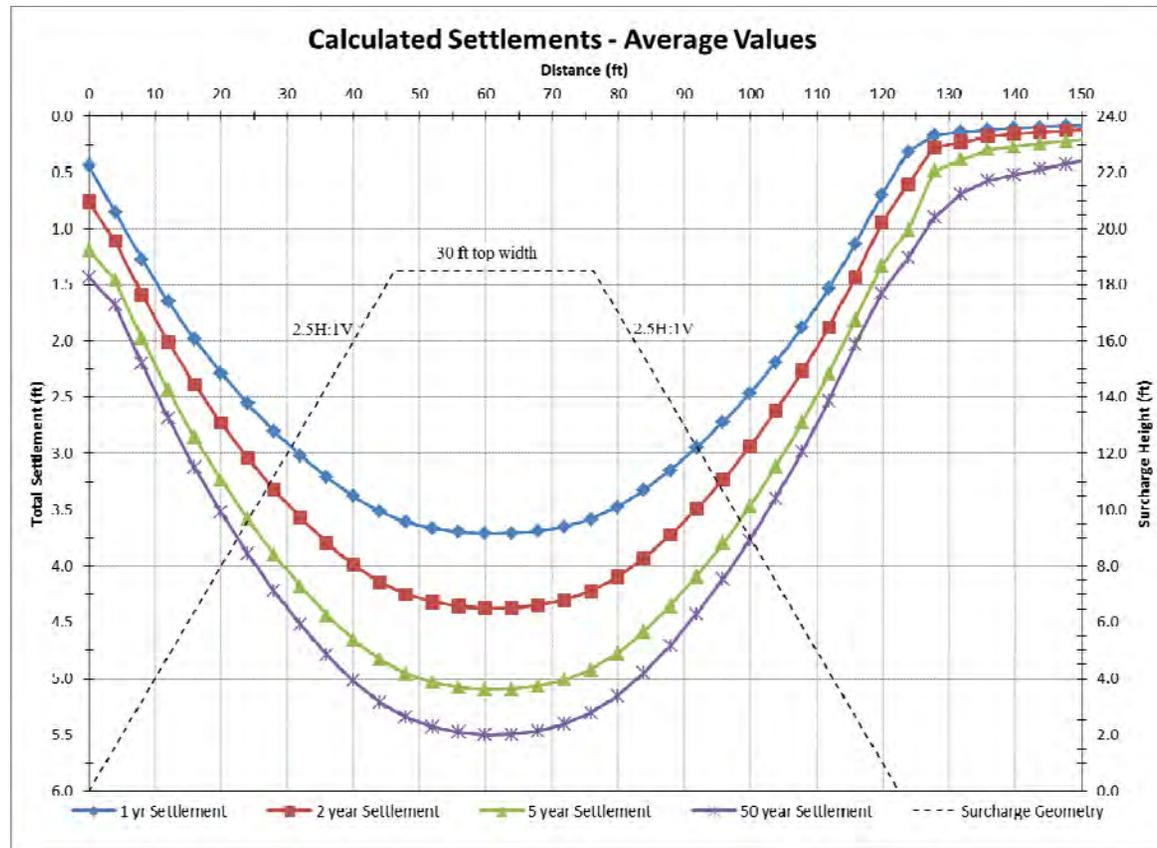
Figure 11. Calculated Primary Consolidation Settlement at Different Times using Average Consolidation Parameters: 18.5- ft Surcharge
