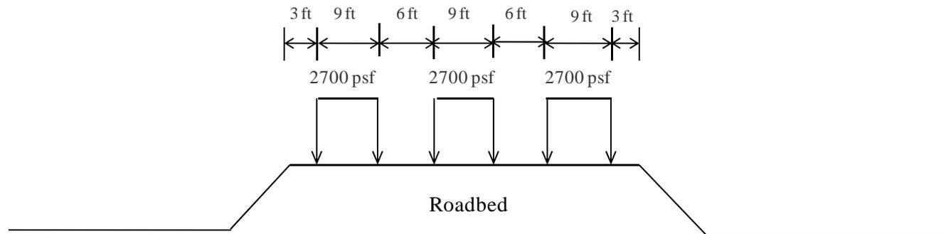
Figure 1. Configuration of Railroad Loading
