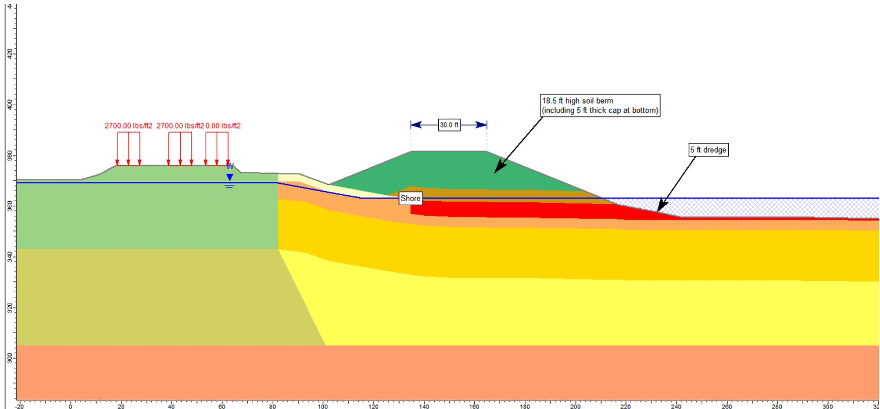
Figure 1B. Stage 2 of Surcharge Placement Sequence: Dredging in front of Soil Berm at Year 2
