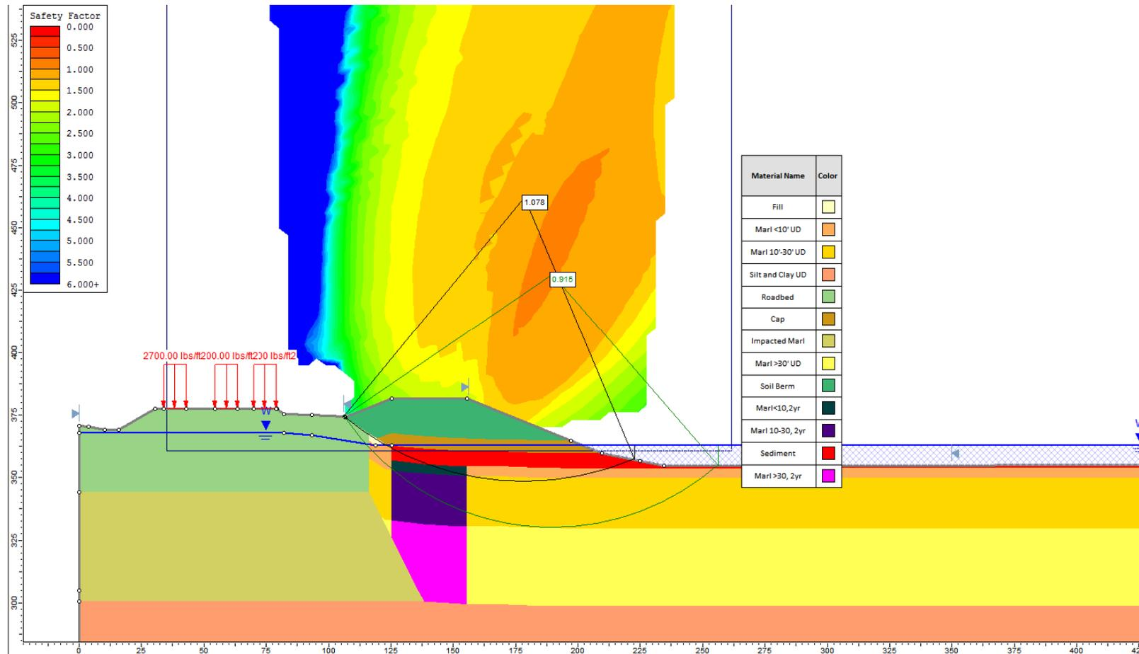
Figure 7. Slope Stability Analysis Results – 18.5-ft Surcharge, Section E5, Stage 2
