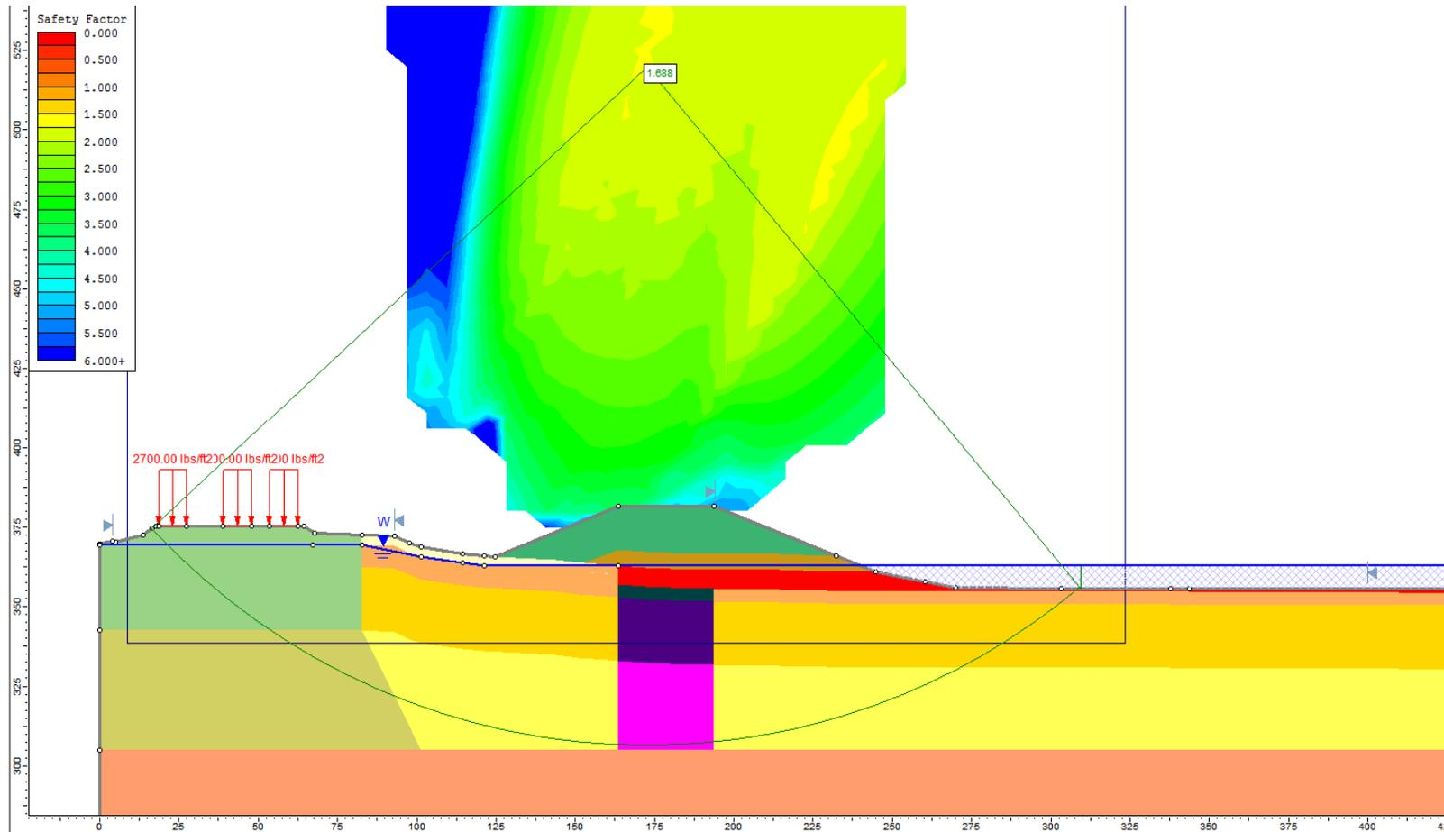
Figure 5. Slope Stability Analysis Results – 18.5-ft Surcharge, Section E3, Stage 2
