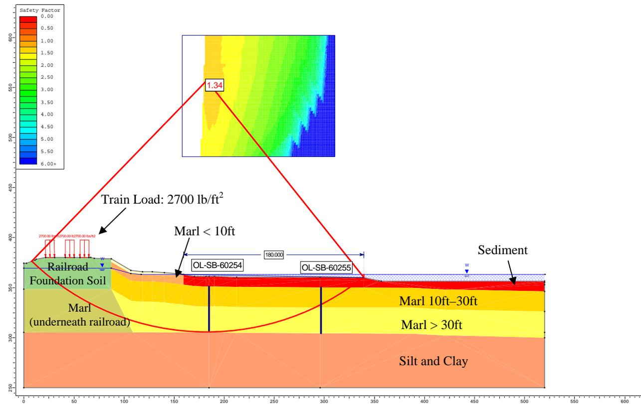
Figure 9. Geometry and Slope Stability Analysis Results of Cross Section E6 (with Offset Distance of 180 ft from the Shoreline)
