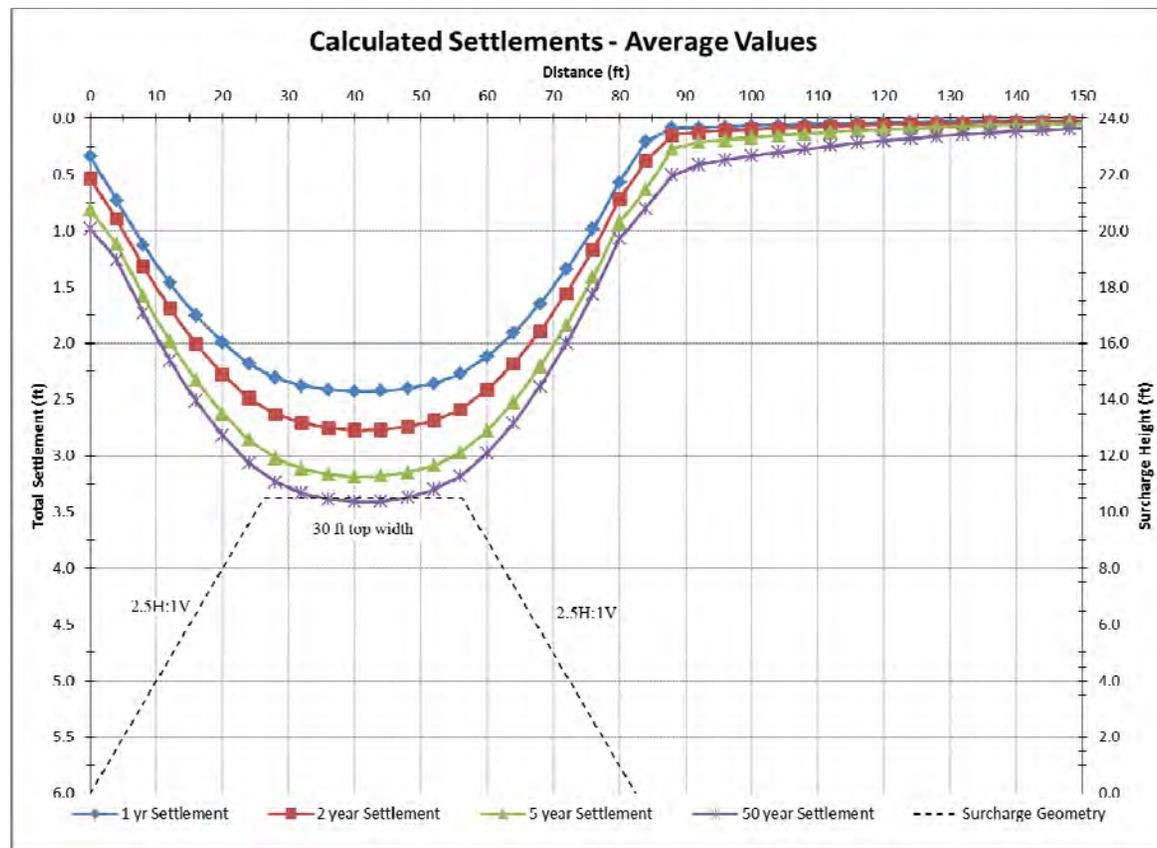
Figure 12. Calculated Primary Consolidation Settlement at Different Times using Average Consolidation Parameters: 10.5- ft Surcharge
