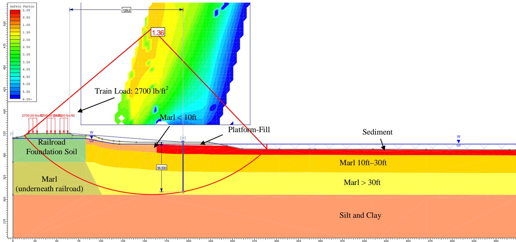
Figure 4. Geometry and Slope Stability Analysis Results of Cross Section E3 where sheetpile is 30 ft away from the shoreline
