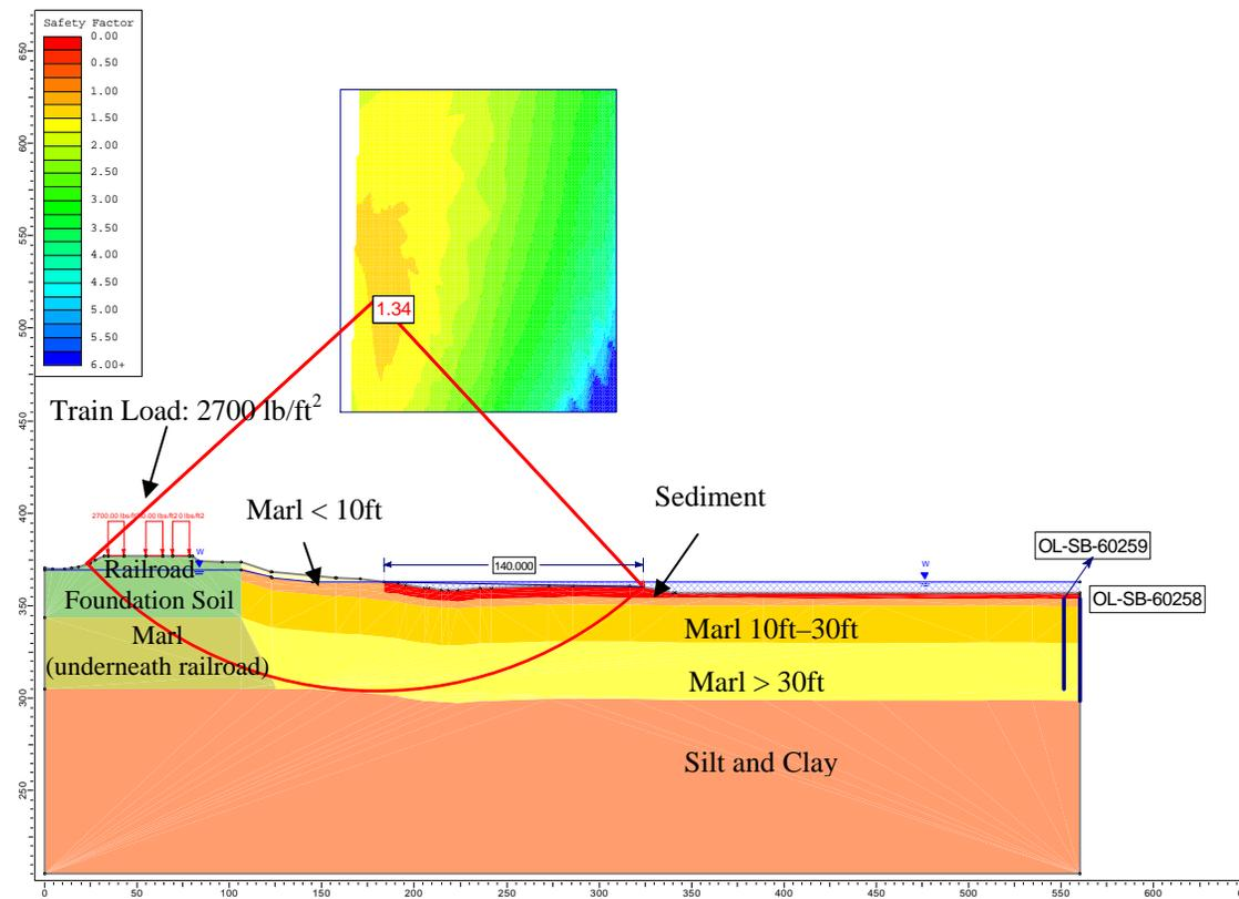
Figure 7. Geometry and Slope Stability Analysis Results of Cross Section E4 (with Offset Distance of 140 ft from the Shoreline)
