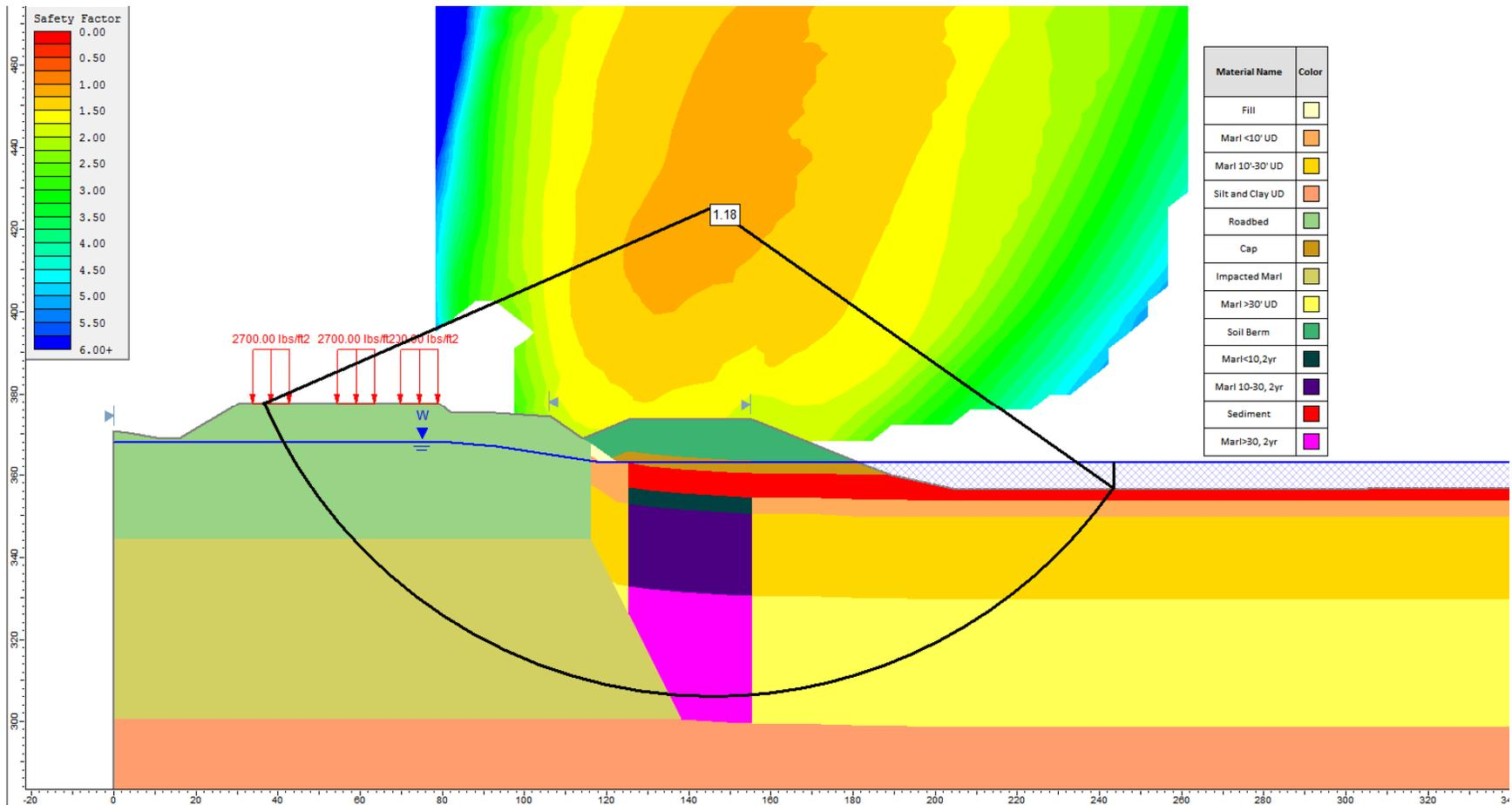
Figure 10. Slope Stability Analysis Results – 10.5-ft Surcharge, Section E5, Stage 2
