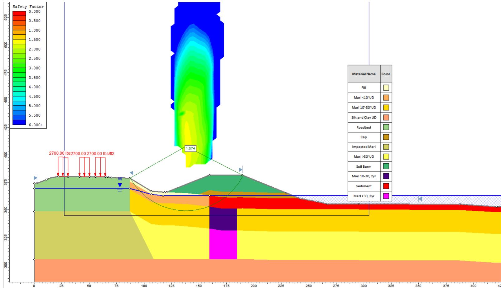
Figure 8. Slope Stability Analysis Results – 18.5-ft Surcharge, Section E6, Stage 2
