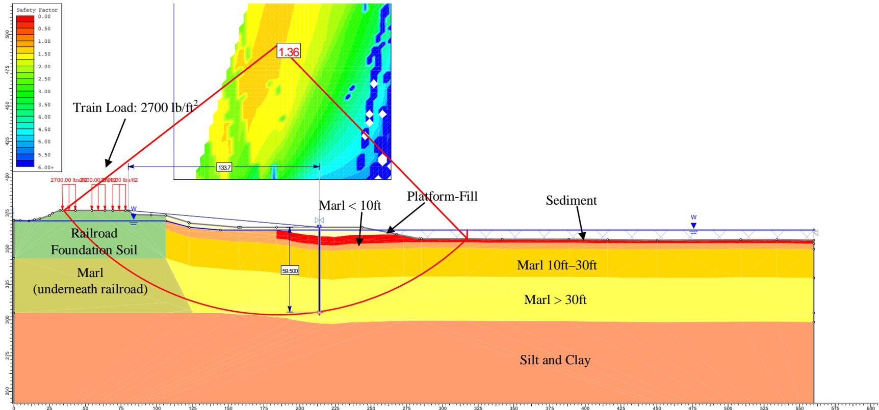
Figure 5. Geometry and Slope Stability Analysis Results of Cross Section E4 where sheetpile is 30 ft away from the shoreline
