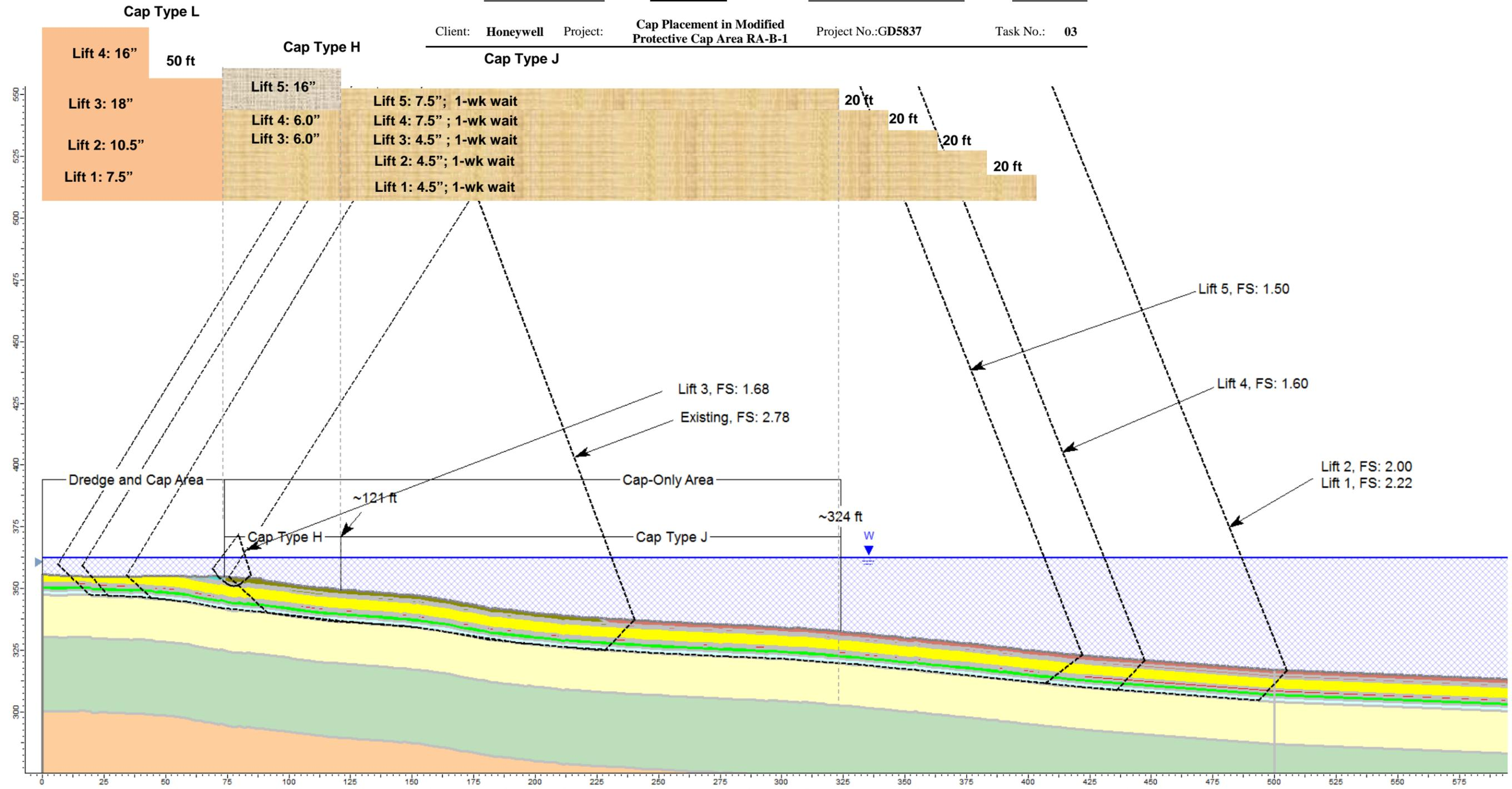
Figure 13. Calculated factors of safety and critical slip surfaces in Cross Section E for various cap placement conditions
