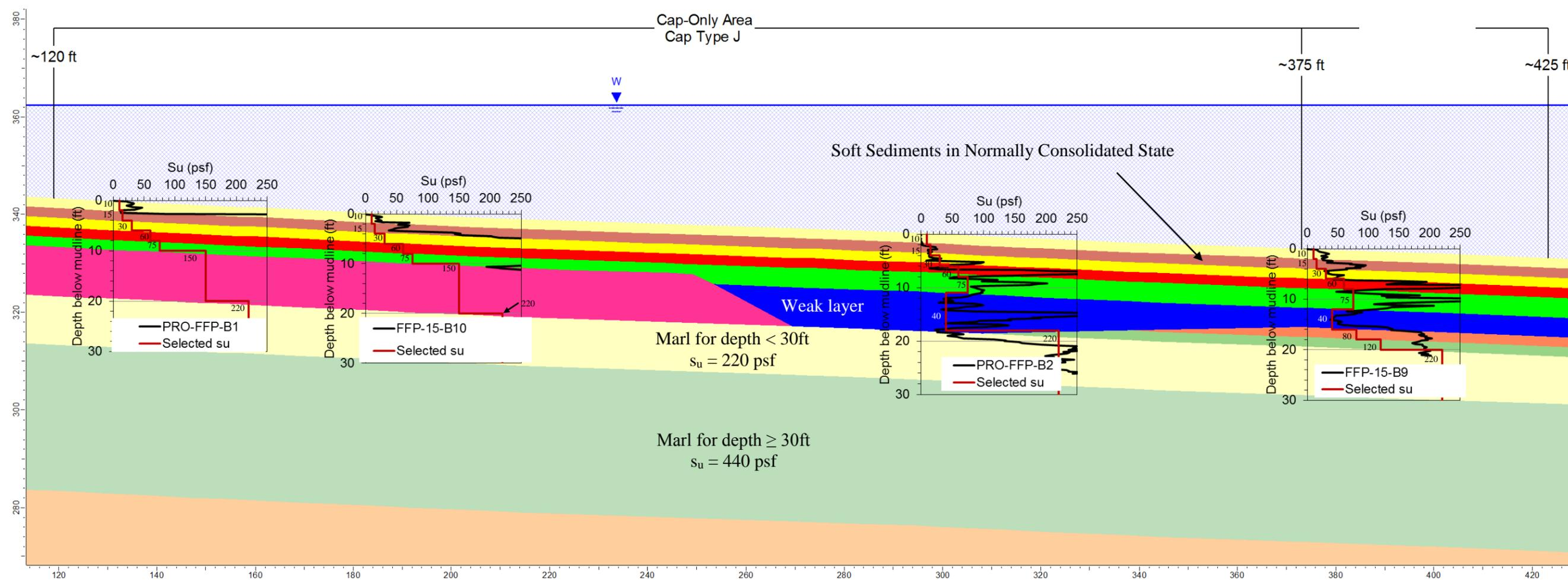
Figure 3. Subsurface stratigraphy and shear strength ( $s_u$ ) profiles from the FFPs collected near Cross Section A. The values on the profiles show the selected shear strengths in psf.
