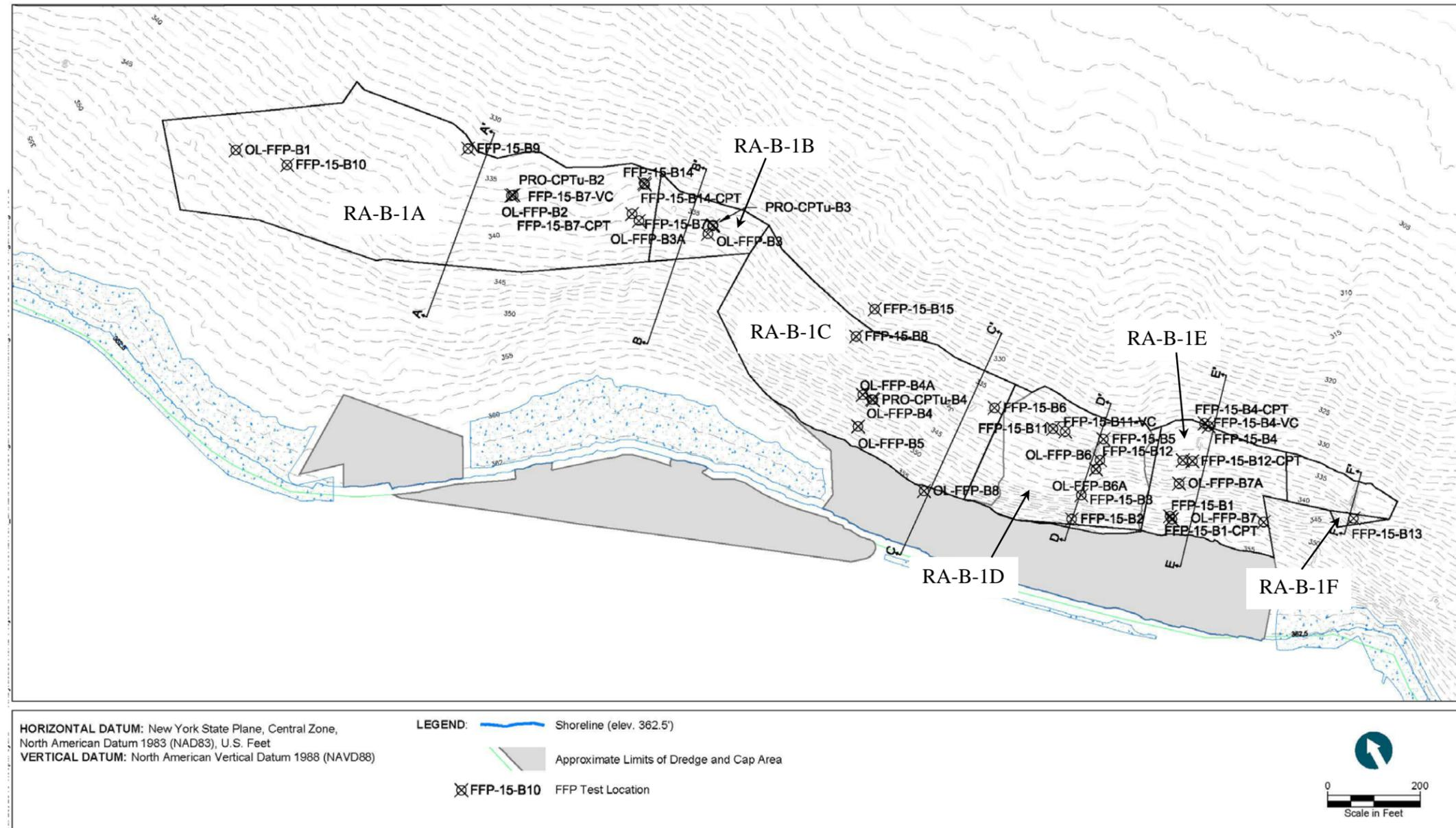
Figure 2. Map of modified protective cap area RA-B-1. This map also shows locations of in situ FFP and CPT tests and the six analyzed cross sections.
