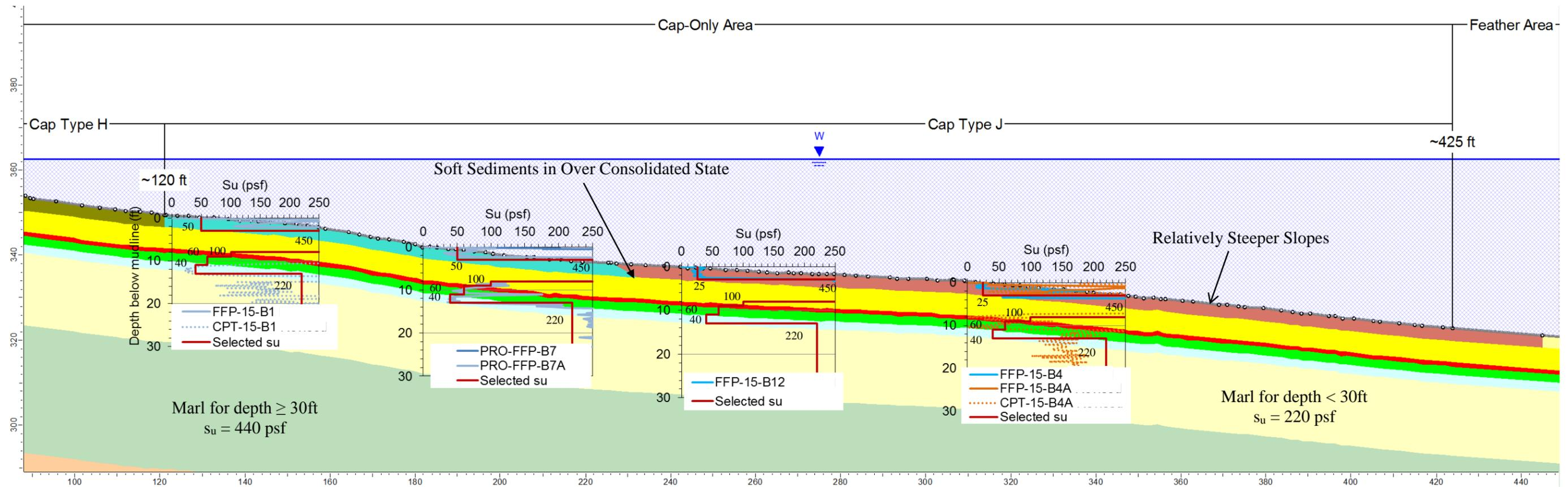
Figure 7. Subsurface stratigraphy and shear strength ( $s_u$ ) profiles from the FFPs collected near Cross Section E
