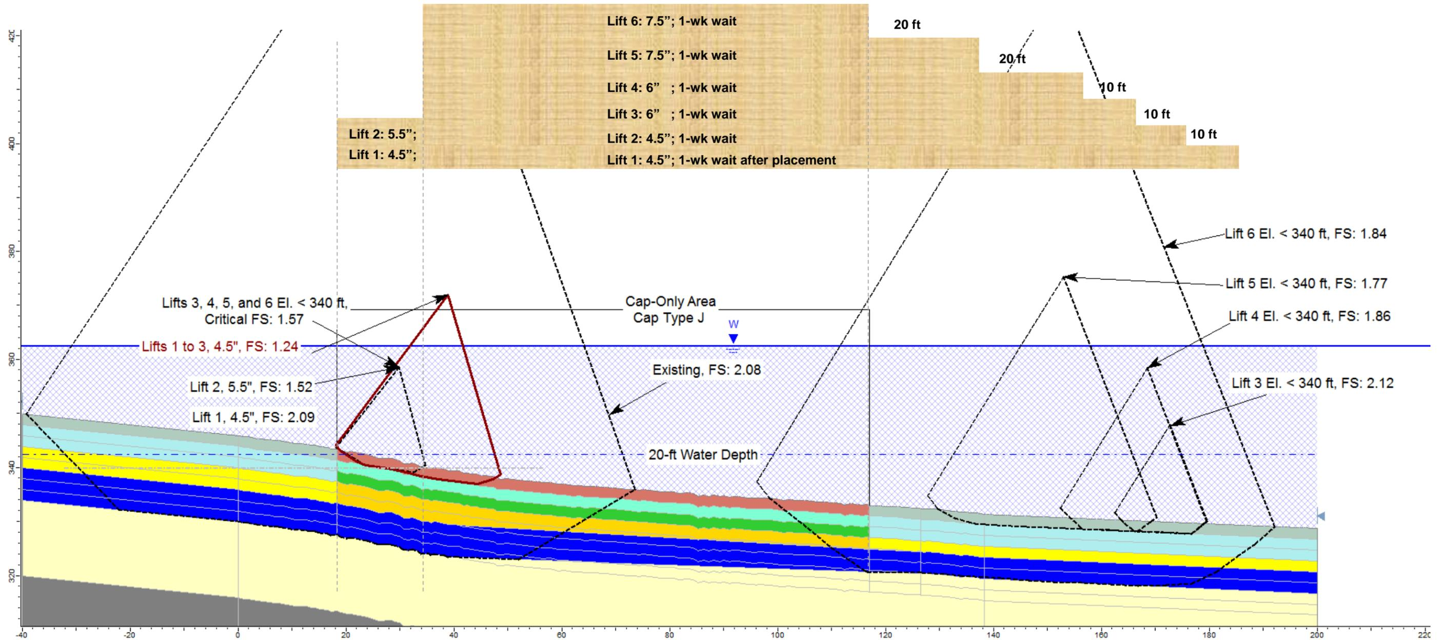
Figure 14. Calculated factors of safety and critical slip surfaces in Cross Section F for various cap placement conditions
