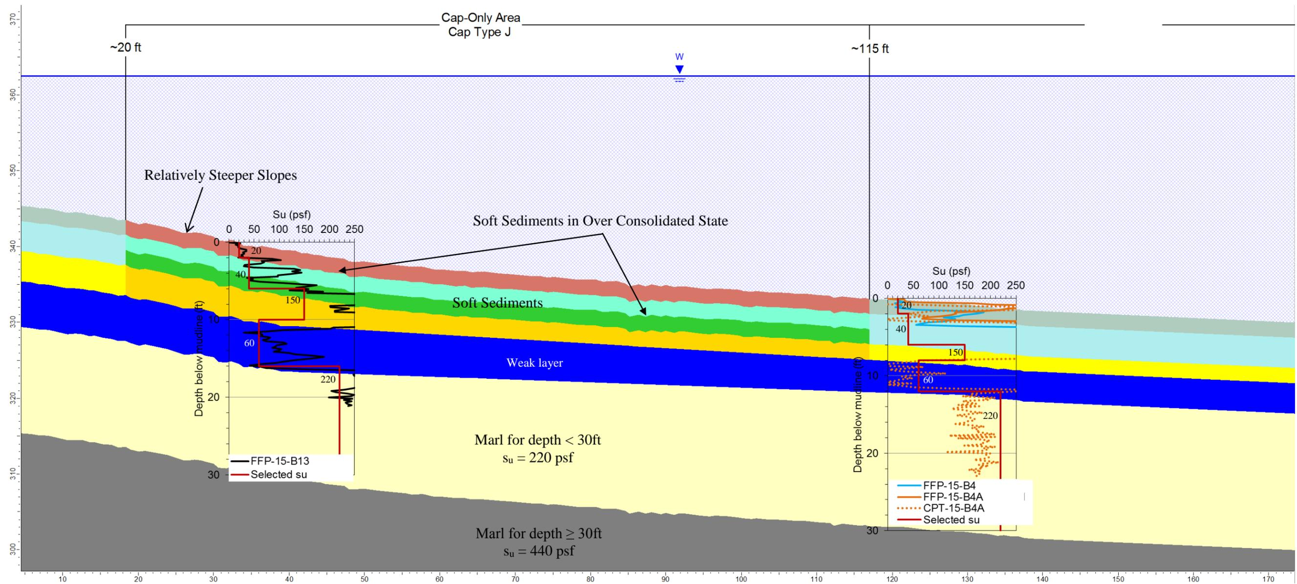
Figure 8. Subsurface stratigraphy and shear strength ( $s_u$ ) profiles from the FFPs collected near Cross Section F
