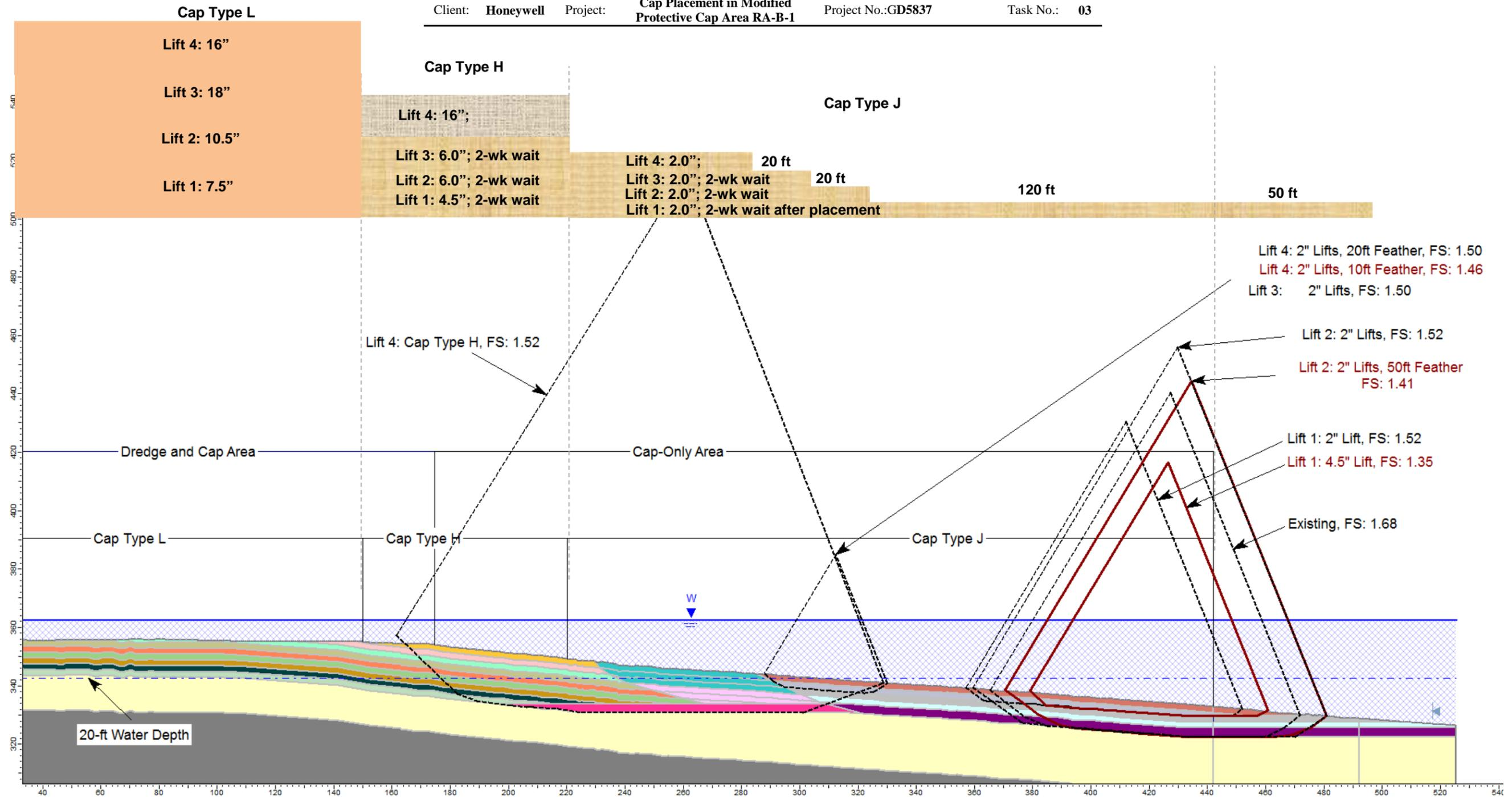
Figure 11. Calculated factors of safety and critical slip surfaces in Cross Section C for various cap placement conditions
