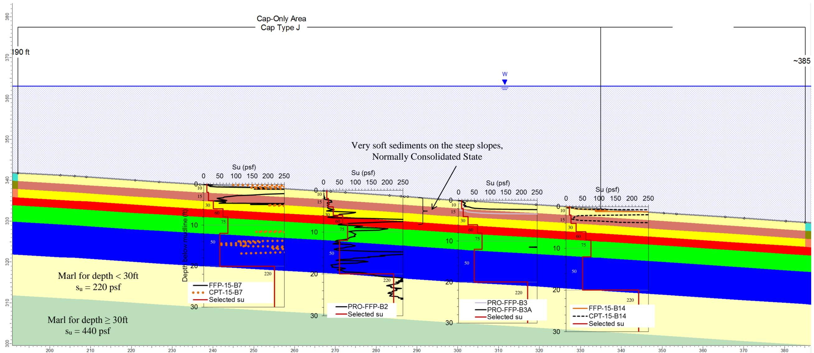
Figure 4. Subsurface stratigraphy and shear strength ( $s_u$ ) profiles from the FFPs collected near Cross Section B
