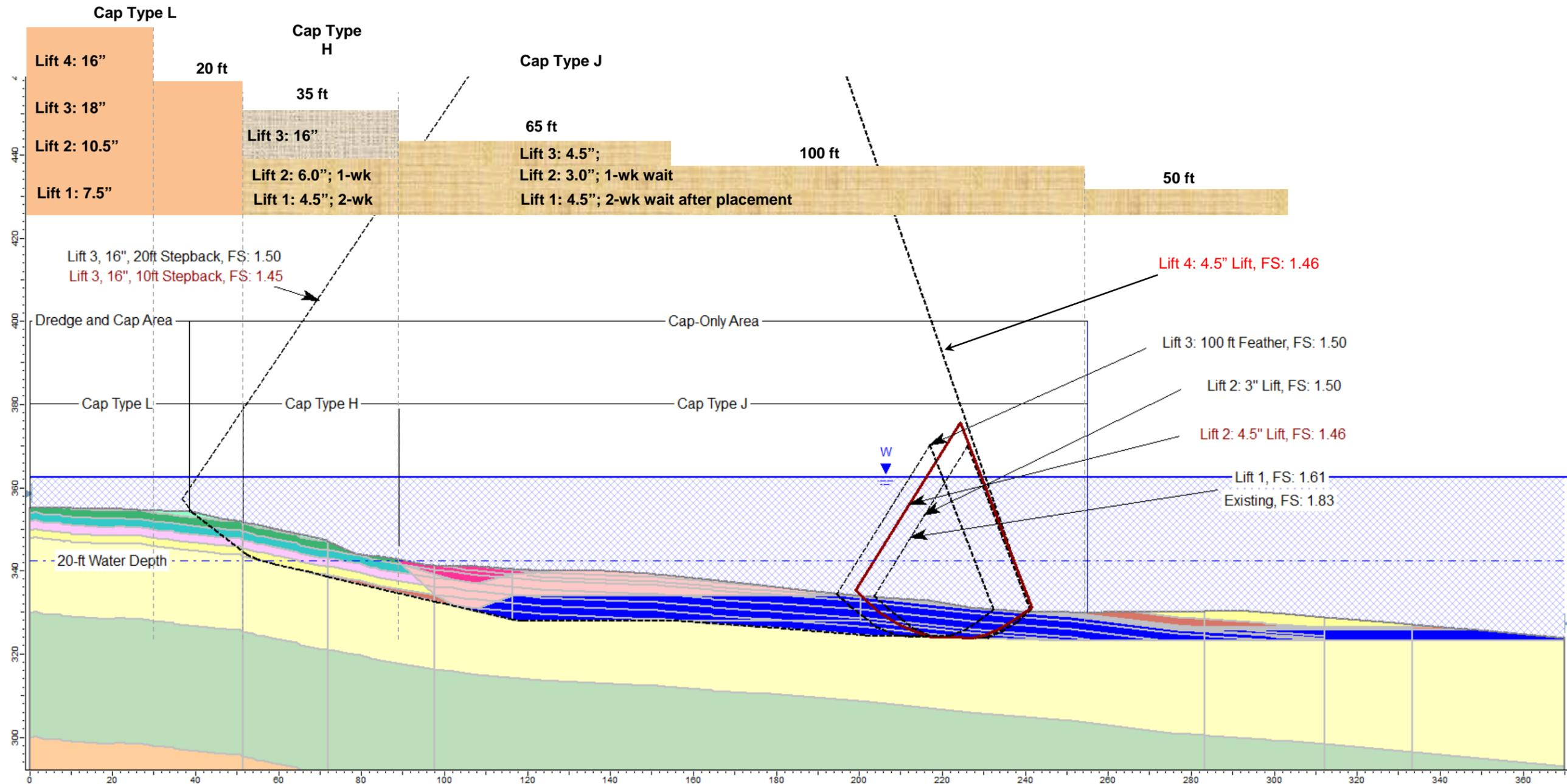
Figure 12. Calculated factors of safety and critical slip surfaces in Cross Section D for various cap placement conditions
