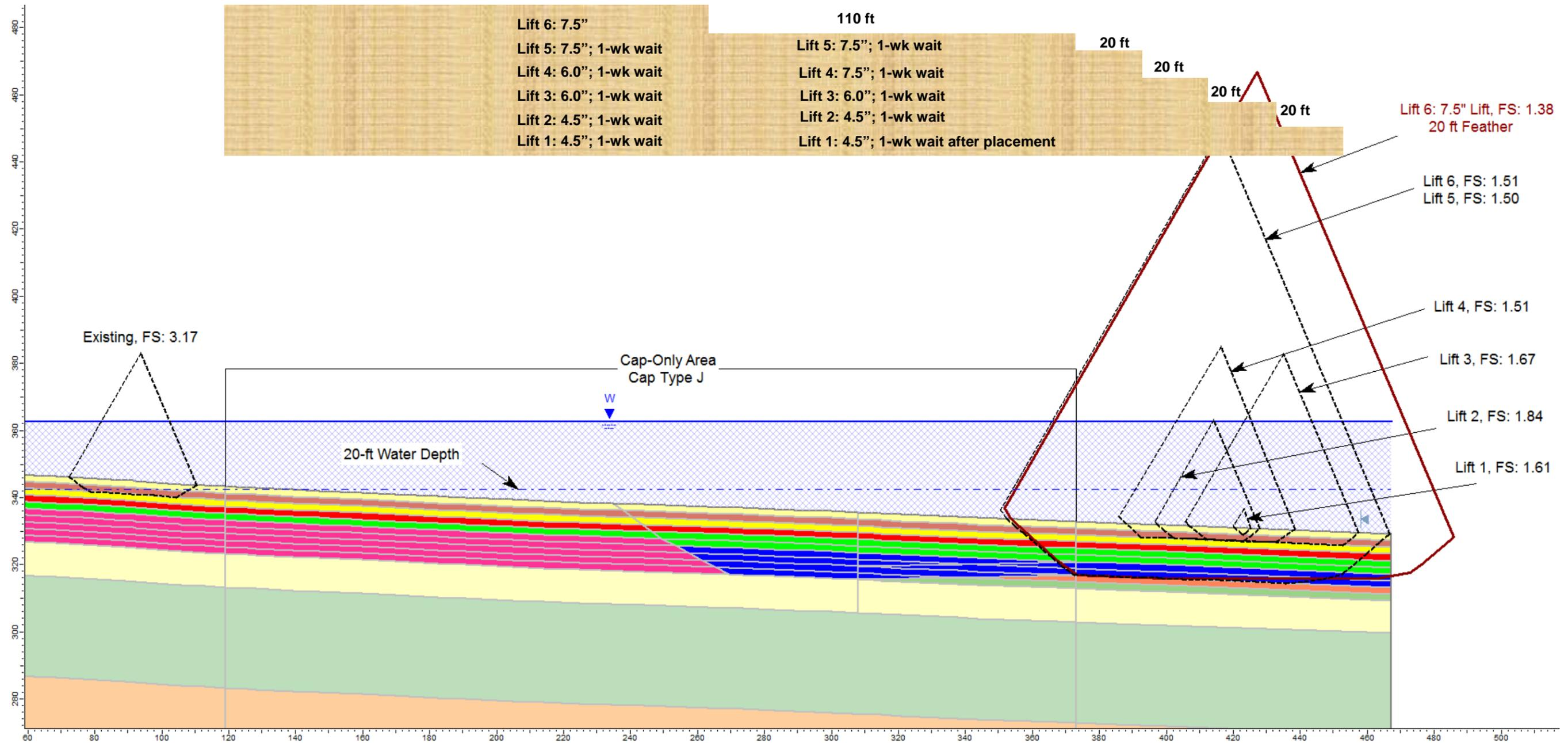
Figure 9. Calculated factors of safety and critical slip surfaces in Cross Section A for various cap placement conditions
