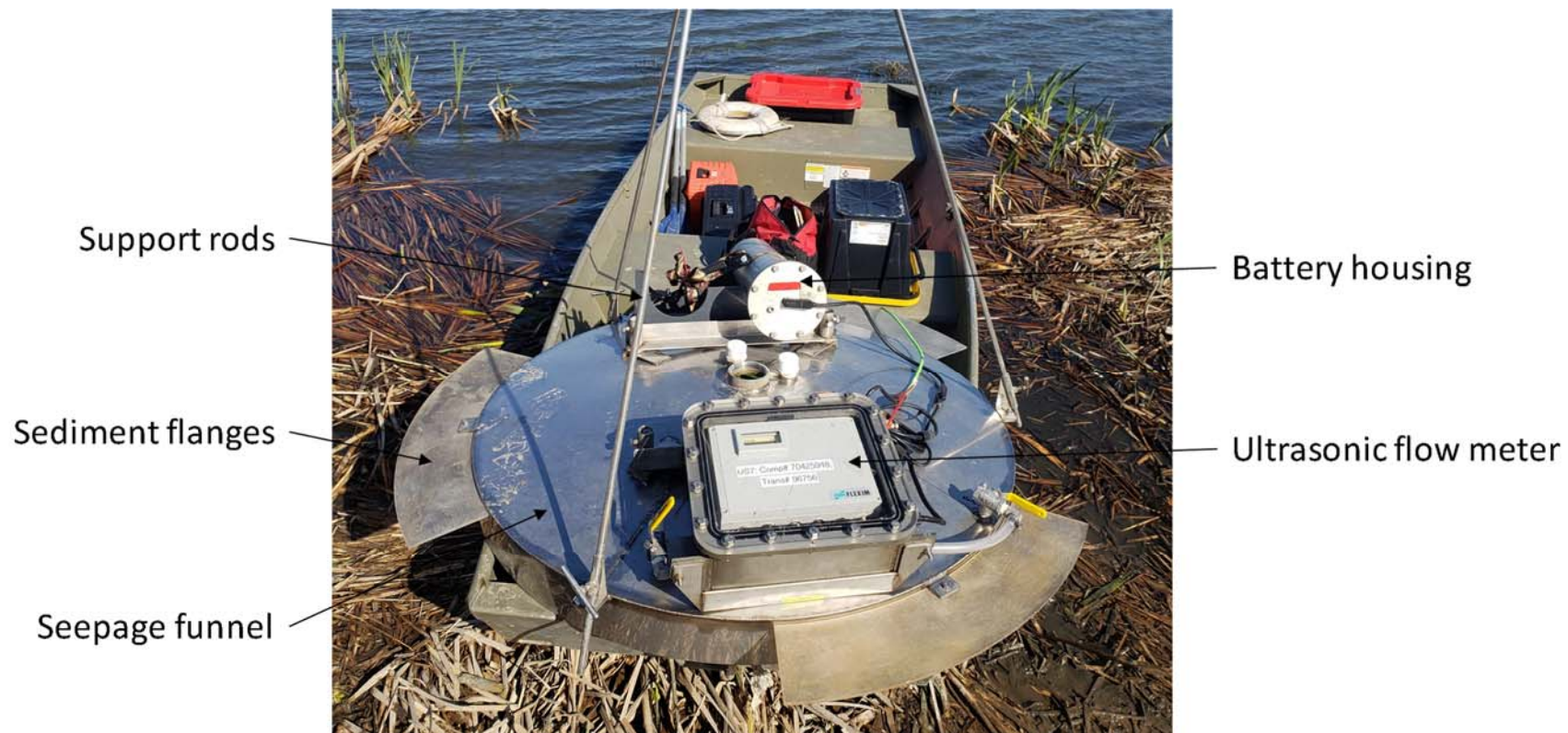
Figure 2-1. The UltraSeep system used to quantify groundwater seepage at the Onondaga Lake site.
