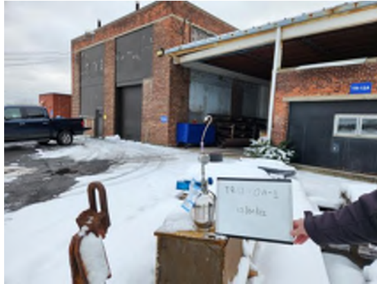
Photo Title: 20221220_085740.jpg Date: 12/20/2022 Description: Outdoor air sample TR12- OA-1
