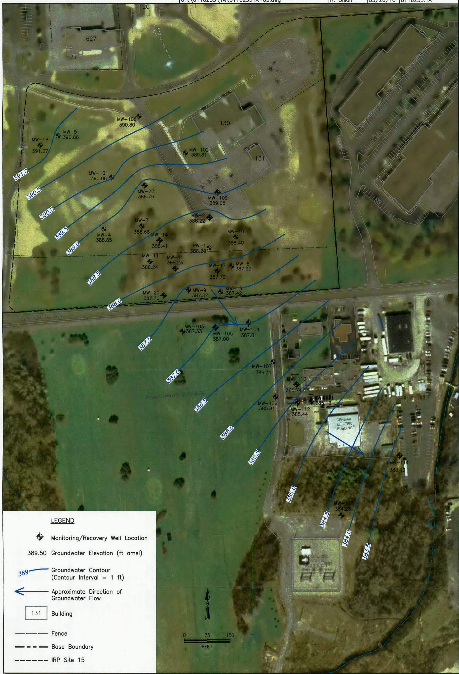
Figure 1-3 Static Groundwater Contour Map 6 October 2009 174th Fighter Wing Hancock Air National Guard Syracuse, New York
