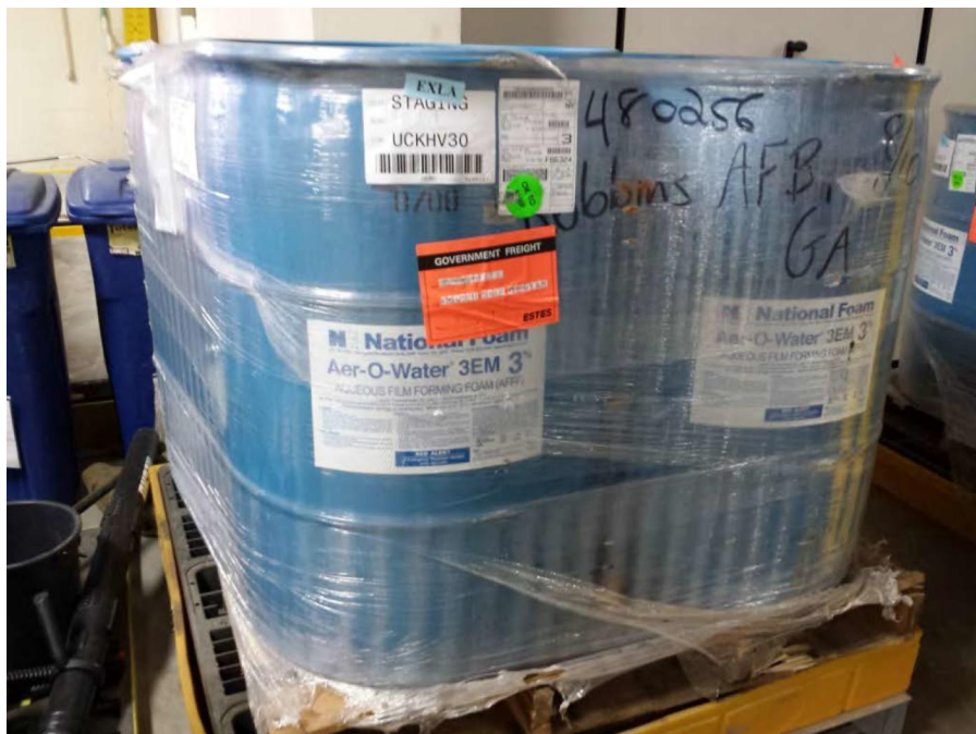
Photo 8: National Foam Aer-O-Water 3EM (3%) AFFF was stored in the Warehouse (Building 614) with secondary containment. No floor drains within the building were observed.
