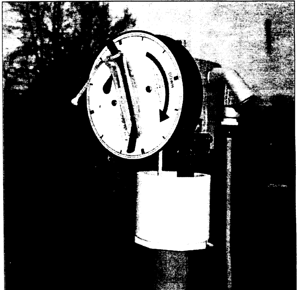
Automatic Level Seek system installed on a 2" PVC wellhead.
