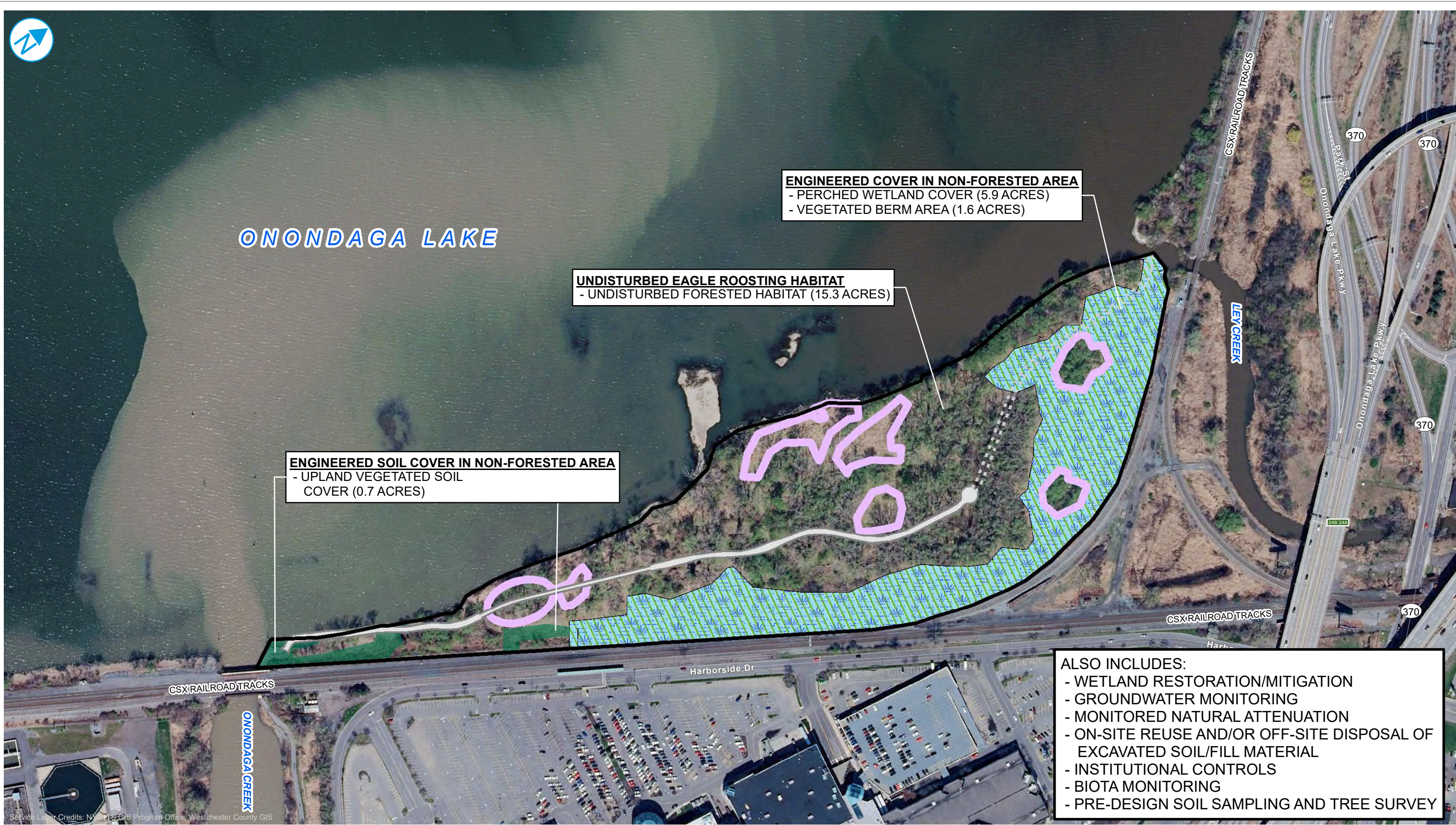
SYW-12 ALTERNATIVE 3 ENGINEERED COVER ON PERIMETER AREA (8.2 ACRES), WETLAND RESTORATION / CREATION, BIOTA MONITORING, AND MNA
