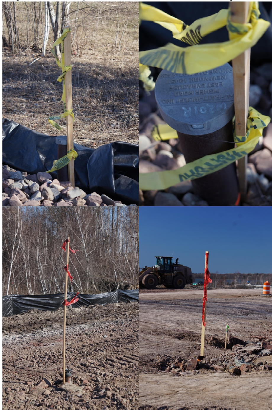
Figure 2-0 Examples of Identified Monitoring Wells
