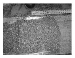
32.5 to 38.0' Sand, medium to Pebbles, coarse; sub-round to sub-angular; trace silt; poor1y sorted; wet; grayish brown (10YR512). NOTE: sedimentary, igneous and metamorphic particles.
