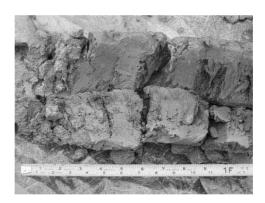
51.4 to 54.0' Clay, some silt, medium to high plasticity, trace small to large pebbles, subround to subangular up to 2" diameter; moist; stiff; dark grayish brown (10YR 4/2) NOTE: Lacustrine ;laminated 0.01 to 0.02 feet thick, laminations brownish yellow (10 YR4/3).
