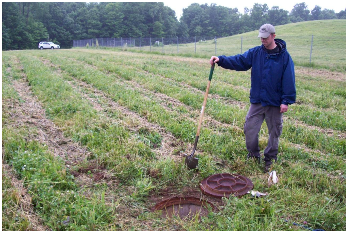
Photo 2: Combination Sampling Sump
