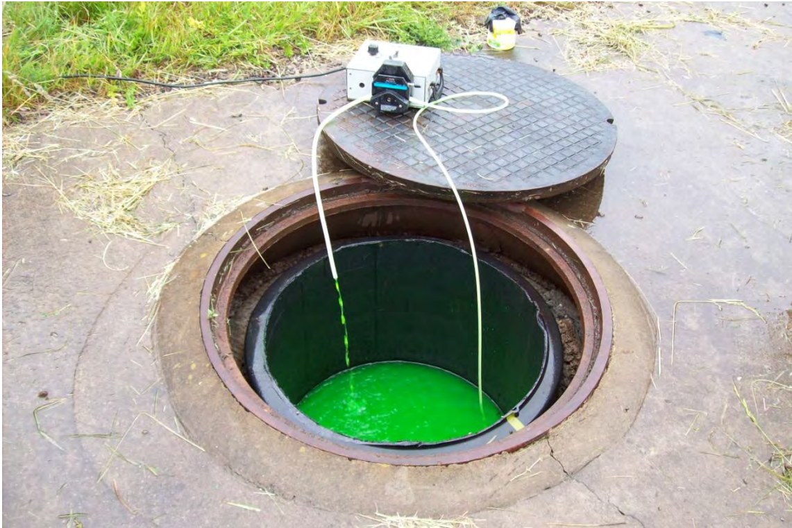
Photo 3: Fluorescent dye in leachate collection tank.
