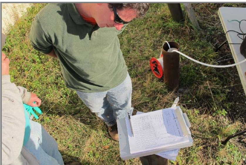
MW-4. Jeremy Wycoff looks at the parameter values of pH, temperature, conductivity, turbidity, etc.
