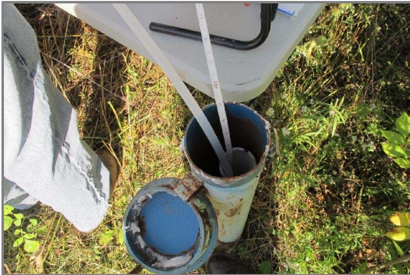
View of MW-7. Coming out of the well are the measuring tape to monitor depth to water and our sampling tubing.
