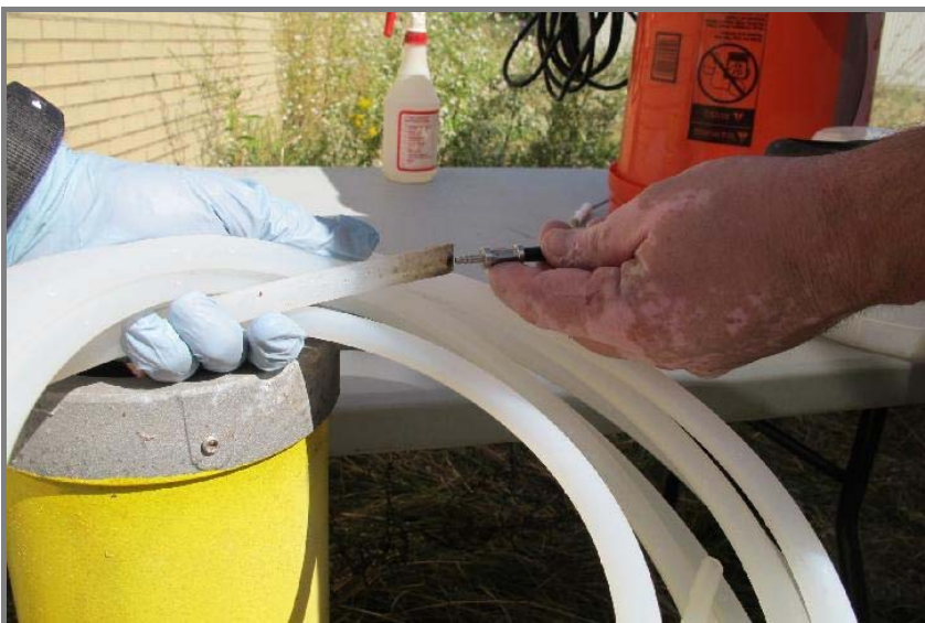
Disposing of the sampling tubing. This well has an oil sheen. The oil is heavier than water and rests at the bottom of the well.
