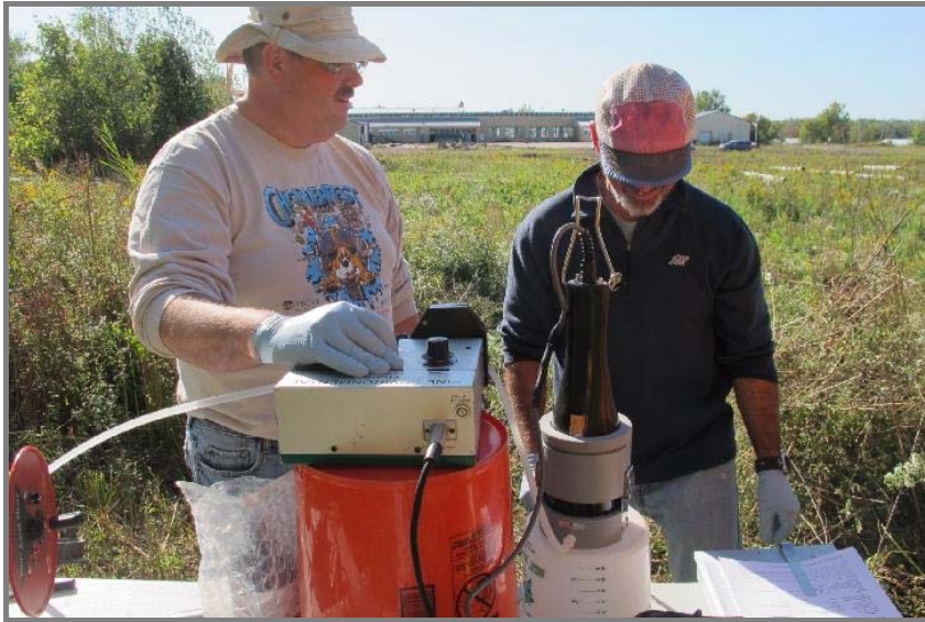
Payson with his hand on the peristaltic sampling pump's on-off switch. Larry reviewing the tally sheets.
