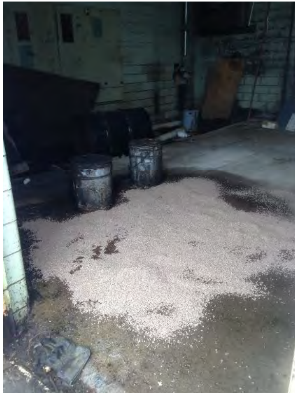
Spill area with absorbent material.
