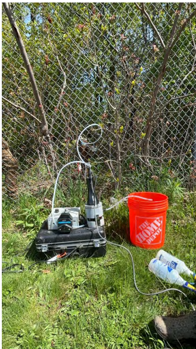
Low-flow groundwater purge setup on MW-6.
