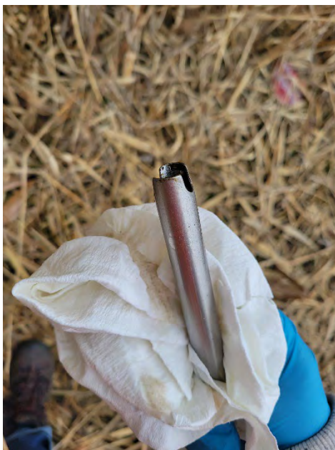
Trace product observed on the oil/water interface probe
