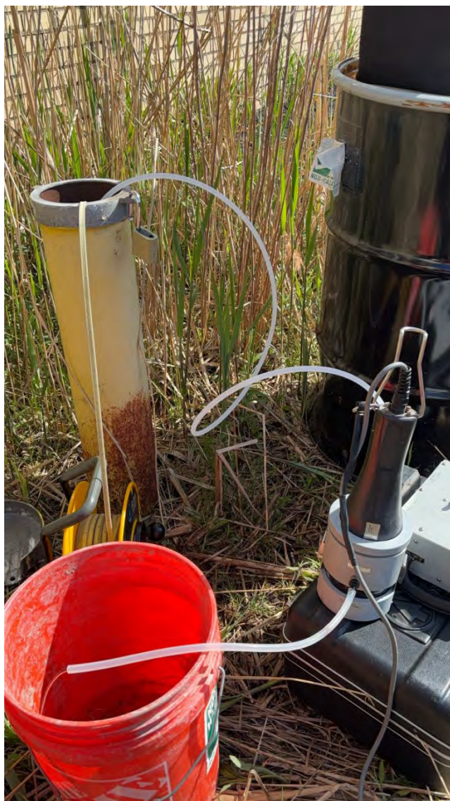
Low-flow groundwater purge setup on MW-1.
