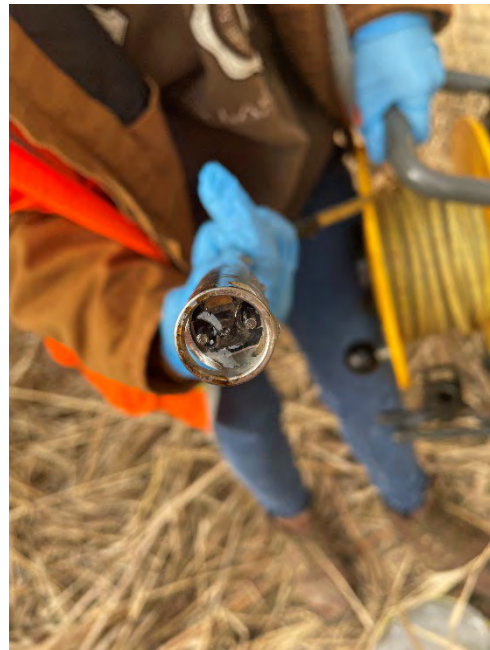
Trace amount of DNAPL present on oil/water probe
