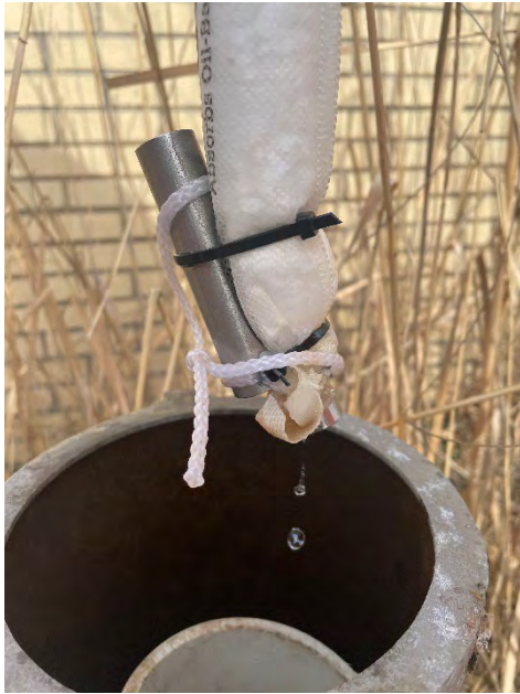
Absorbent sock removed from MW-1 with no visible DNAPL
