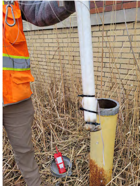
Some product observed on the absorbent sock from MW-1
