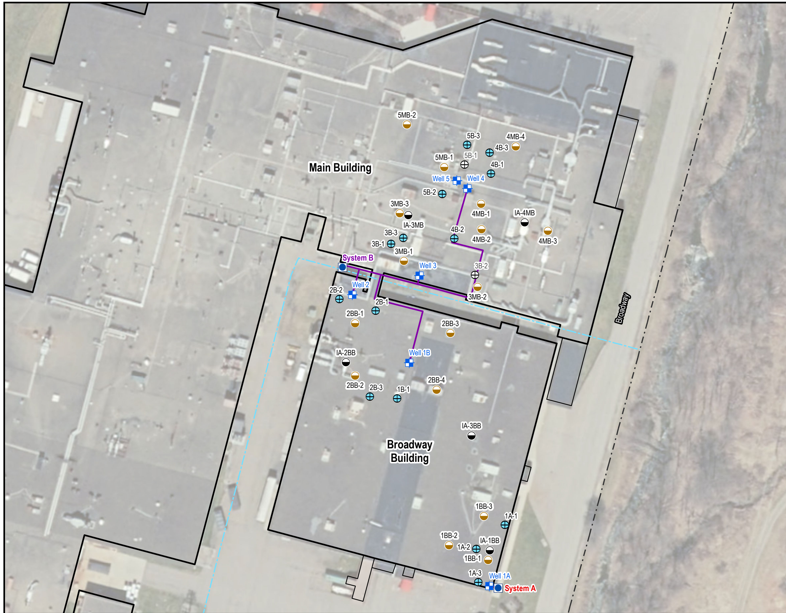
Figure 2: Vapor Intrusion Sample Locations and Sub-Slab Depressurization Monitoring Points Sanmina Owego, NY May 2019
