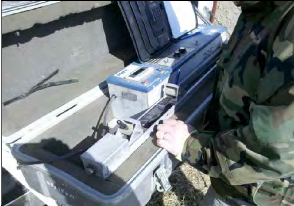
Stress testing the strength of the weld.
