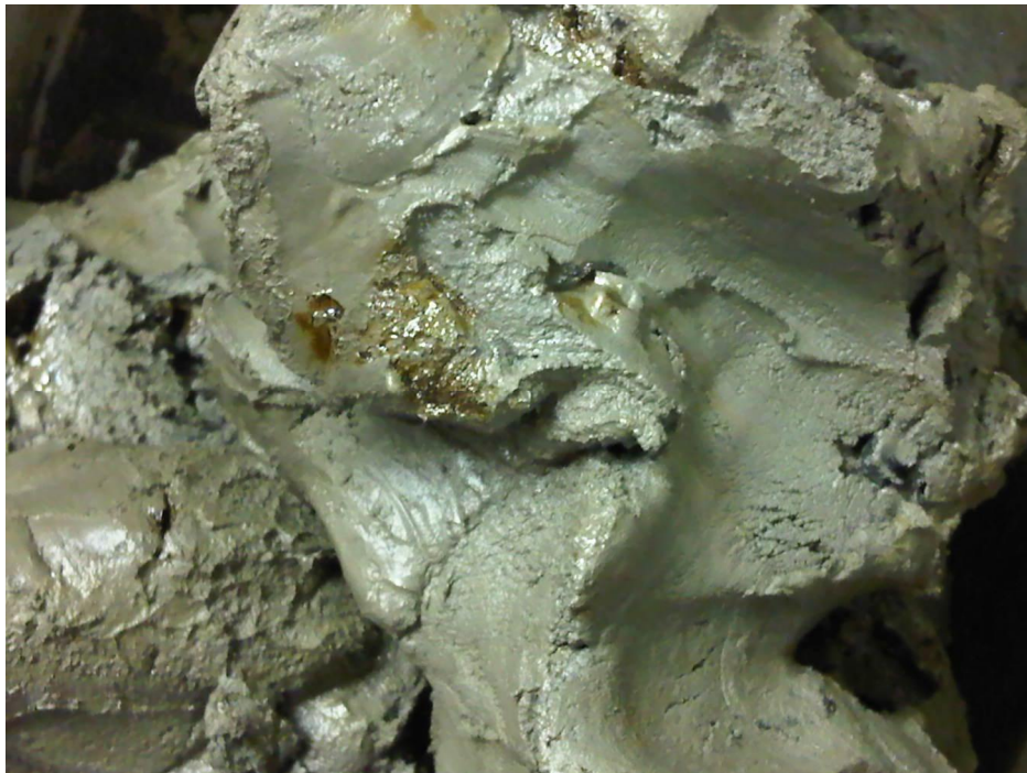
Photograph 2. Non-aqueous phase liquid was observed in field soil samples.
