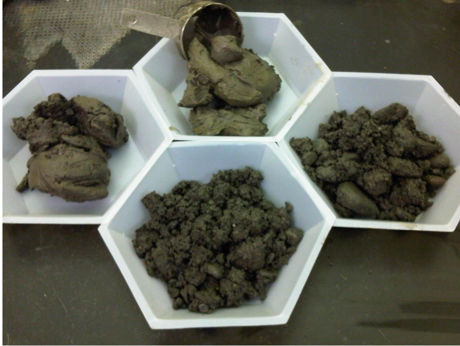
Photograph 1. Field samples provided to the AECOM Treatability Laboratory consisted of a range of soil types including silty clay, sand, and gravel.
