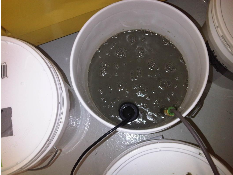
Photograph 3. Due to the large aqueous and soil sample volumes required, Phase II bench scale testing was performed in new five-gallon buckets. Off-gassing of oxygen gas was observed immediately following the addition of hydrogen peroxide to the soil slurry.
