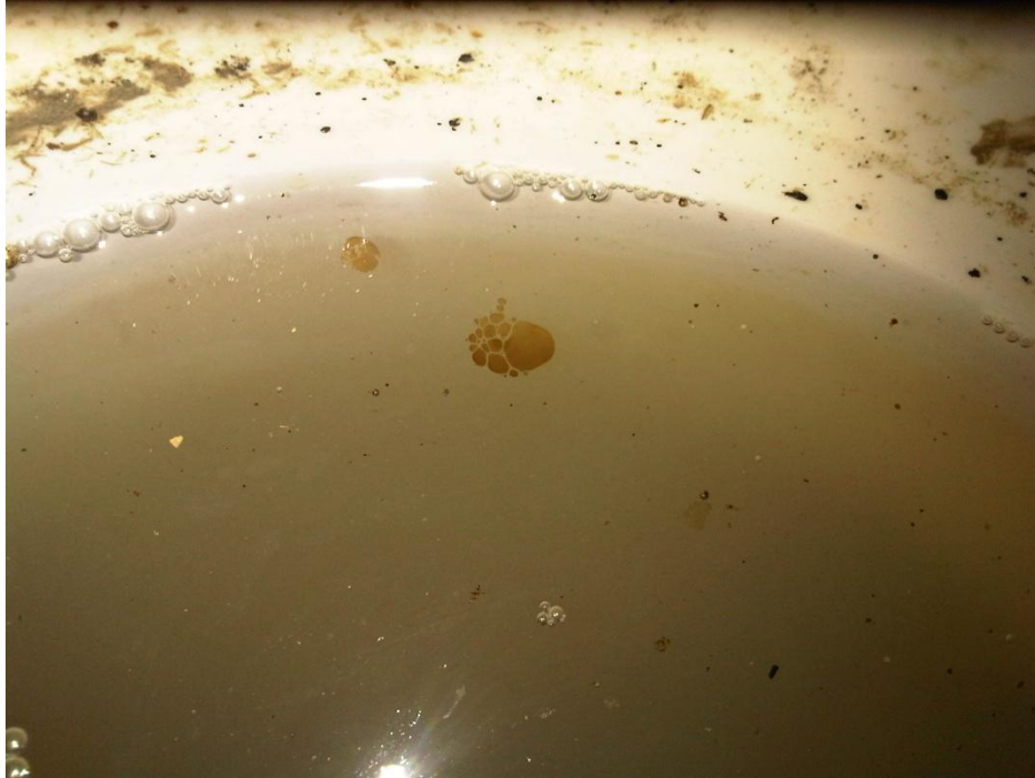
Photograph 4. Non-aqueous phase liquid was observed to be released from the soil after application of hydrogen peroxide during the testing.
