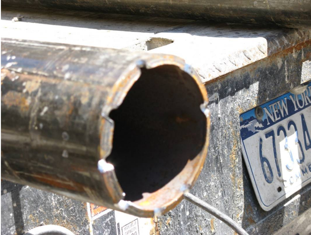
Monitoring Point Bottom - Notched 4" Steel Casing
