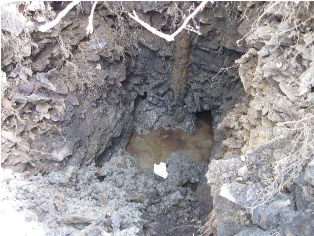
Photograph 26: Petroleum product and groundwater entering the open test pit.
