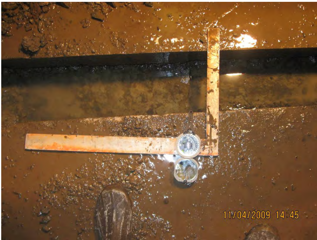
Photograph 16: Measuring the trend of a vertical joint in T-1 (N17W).
