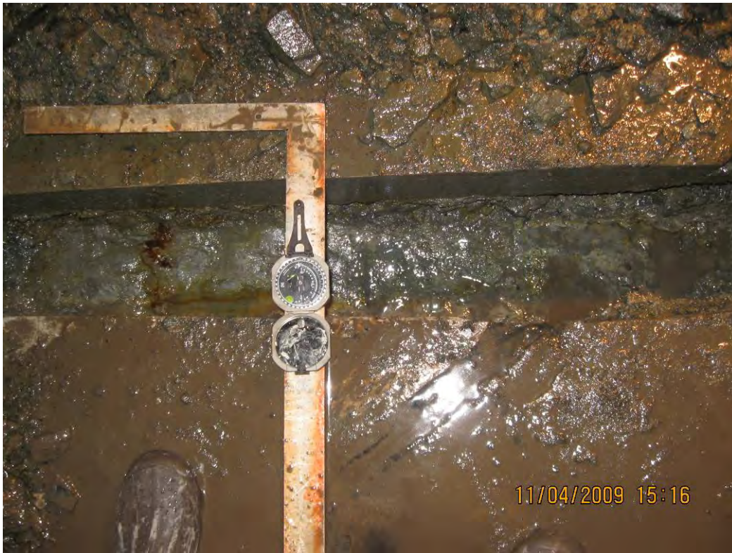
Photograph 19: Measuring the alignment of the vertical fracture producing petroleum product.
