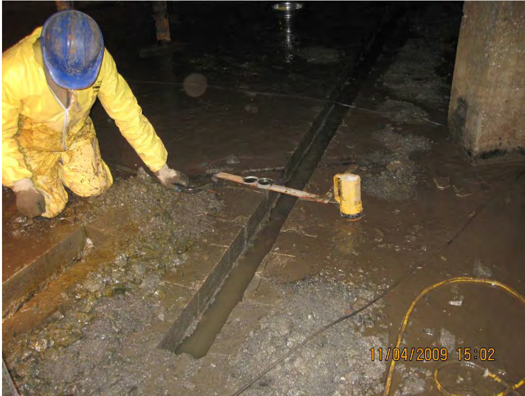
Photograph 18: Measuring the trend of a vertical joint found in T-1.
