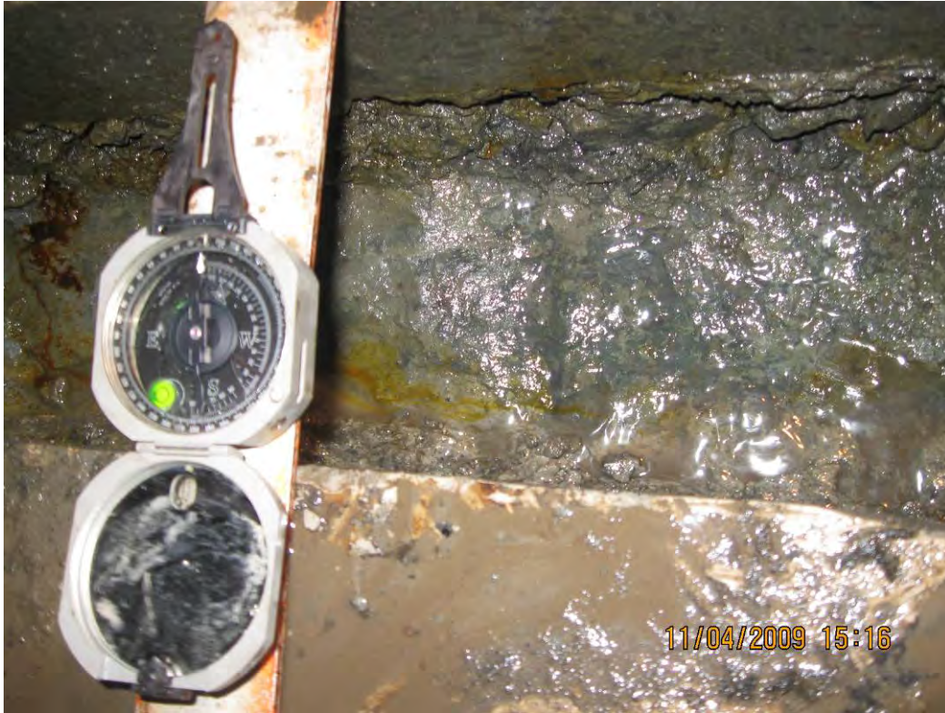
Photograph 20: Measuring the alignment of the vertical fracture producing petroleum product.
