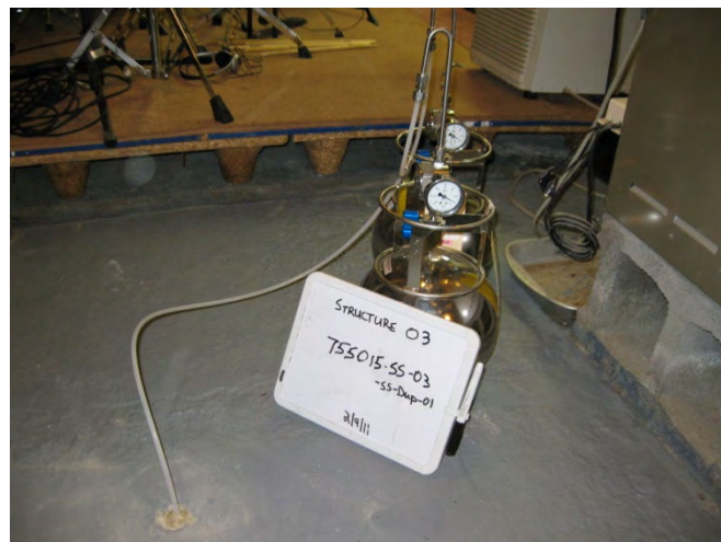
Sub-Slab Sample SS-03 (February – Took in water, suitable sample not collected)
