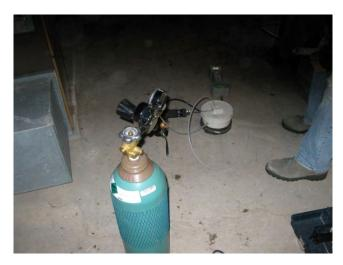
Leak Testing for Sub-Slab Point SS-01
