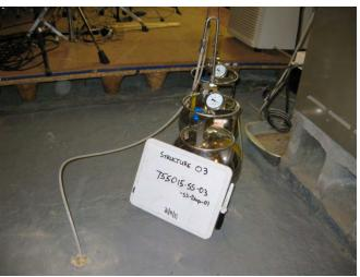
Sub-Slab Sample SS-03 (February – Took in water, suitable sample not collected)
