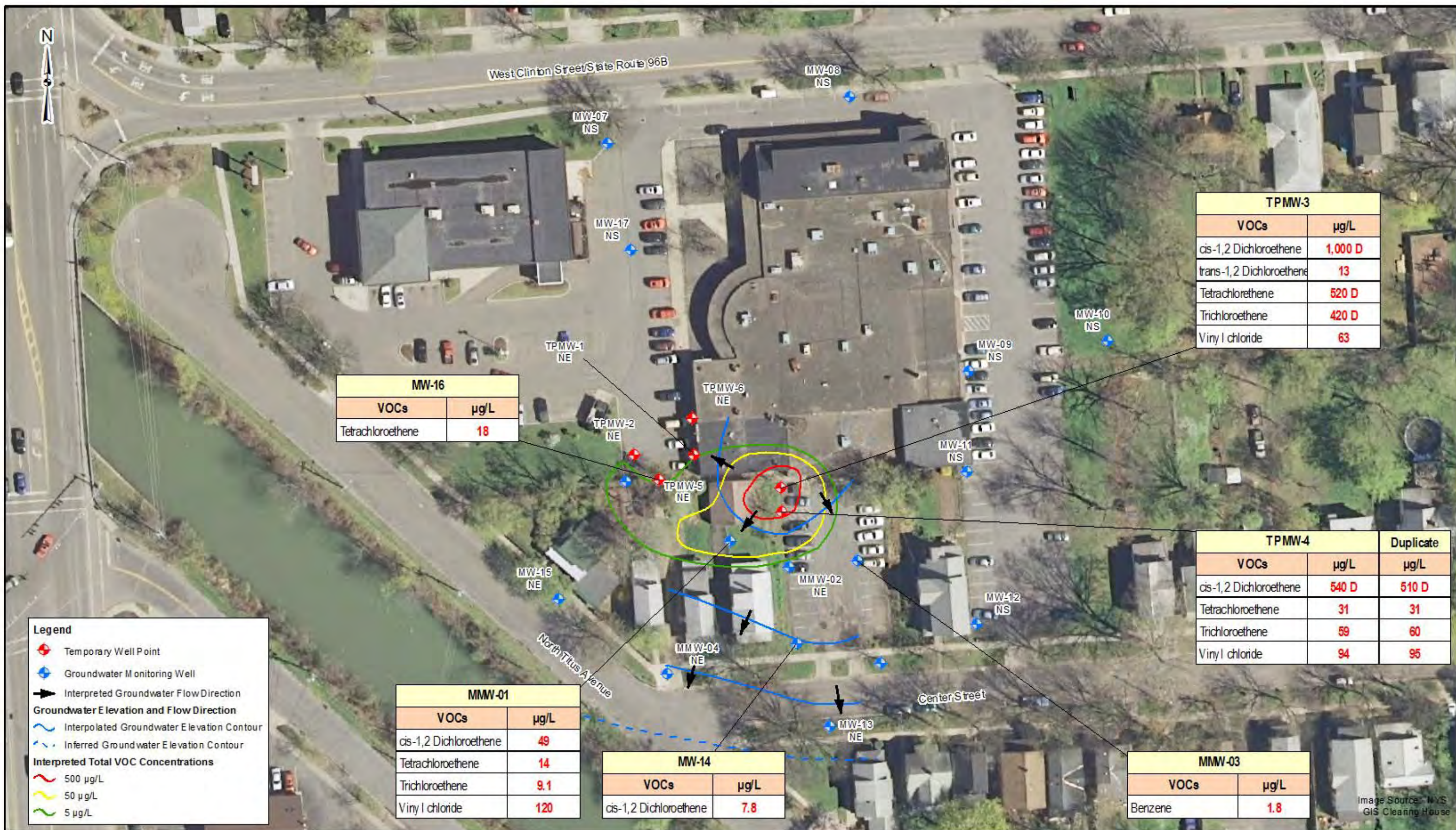
FIGURE 6 Chlorinated Volatile Organic Compounds Detected in Groundwater Samples May 2011
