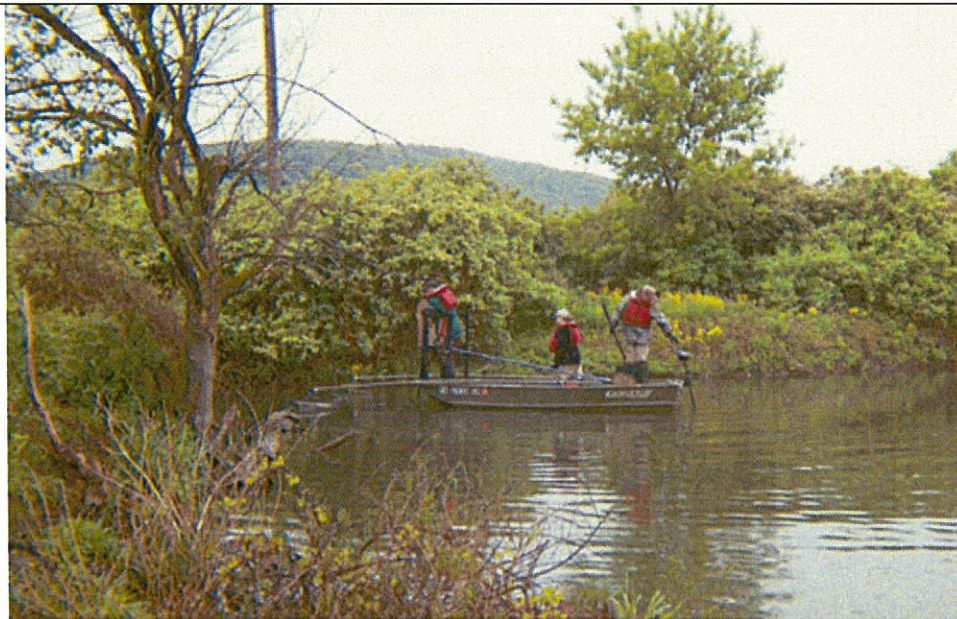
Photo #2 Example of electroshock set-up on the Jon boat.
