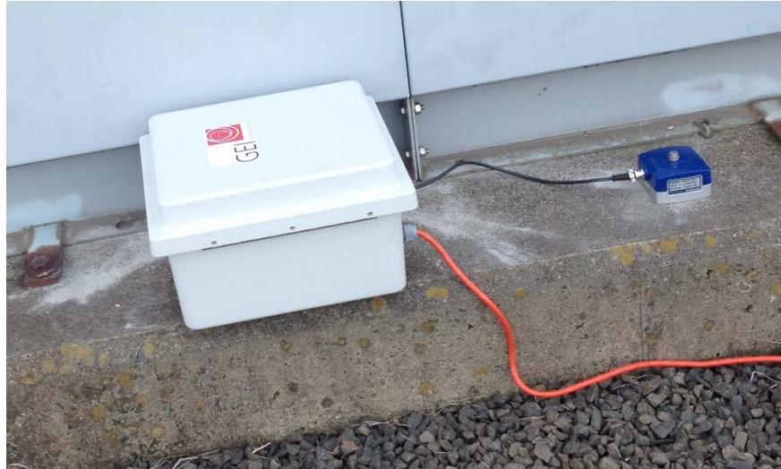
Photo: Typical Seismograph Installation on horizontal surface
