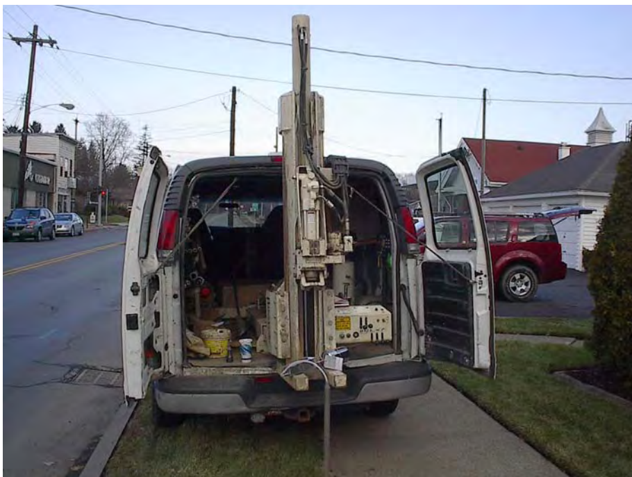
Geoprobe 5400 rig in the process of collecting a soil vapor sample (GV-3).
