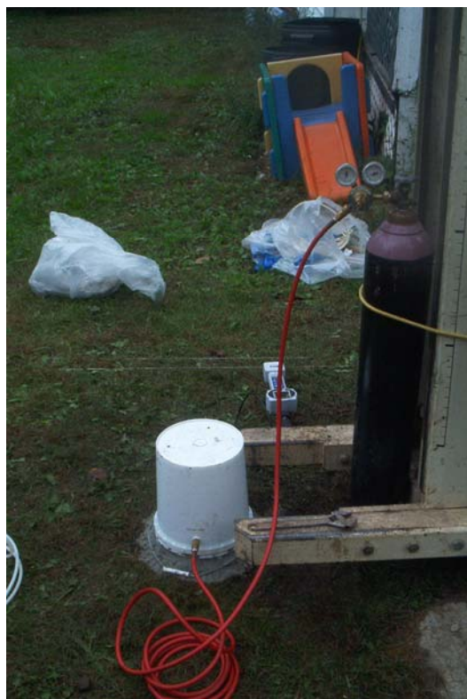
Conducting Helium Breakthrough Test GV-3.
