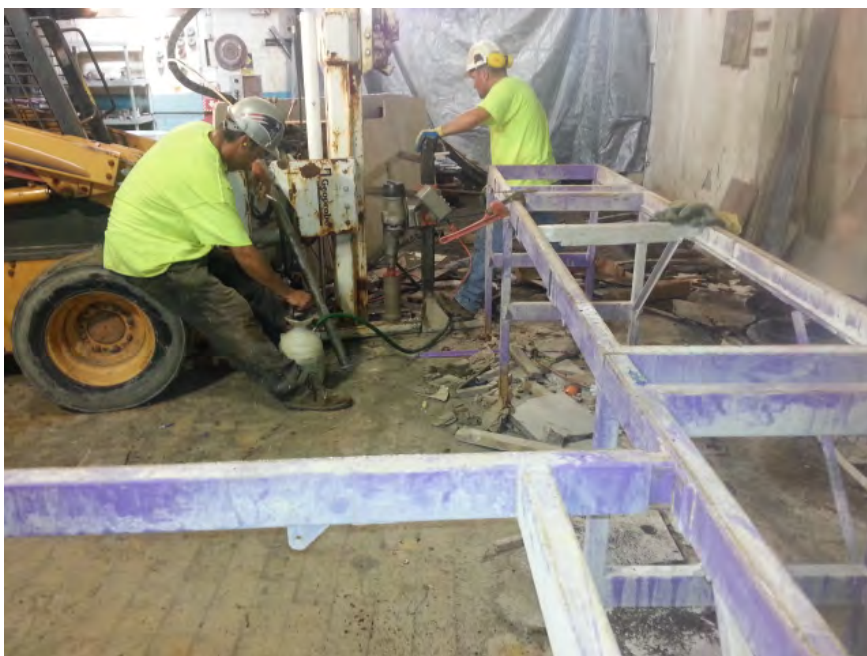
Photo 18: 08/29/13 – Hydraulic direct-push unit (geoprobe) location GS-08.
