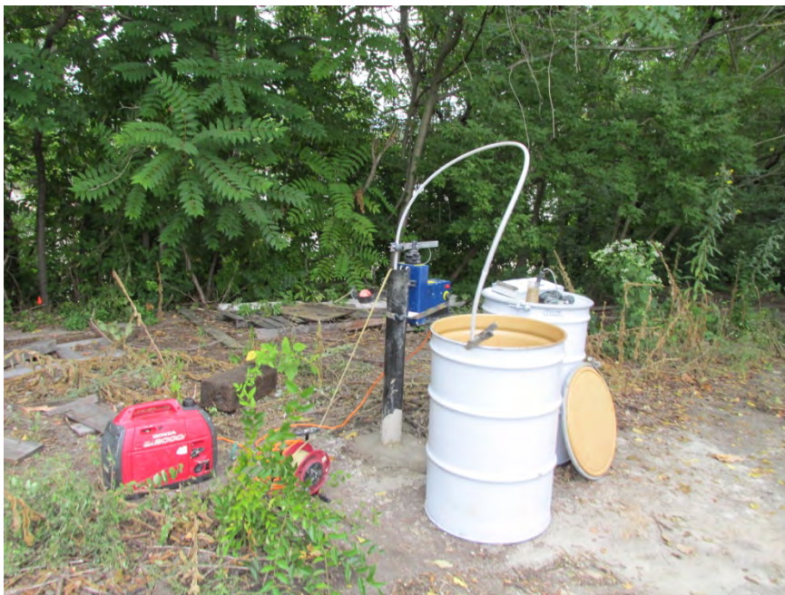
Photo 9: 08/29/13 – Well development at monitoring well location MW-02.
