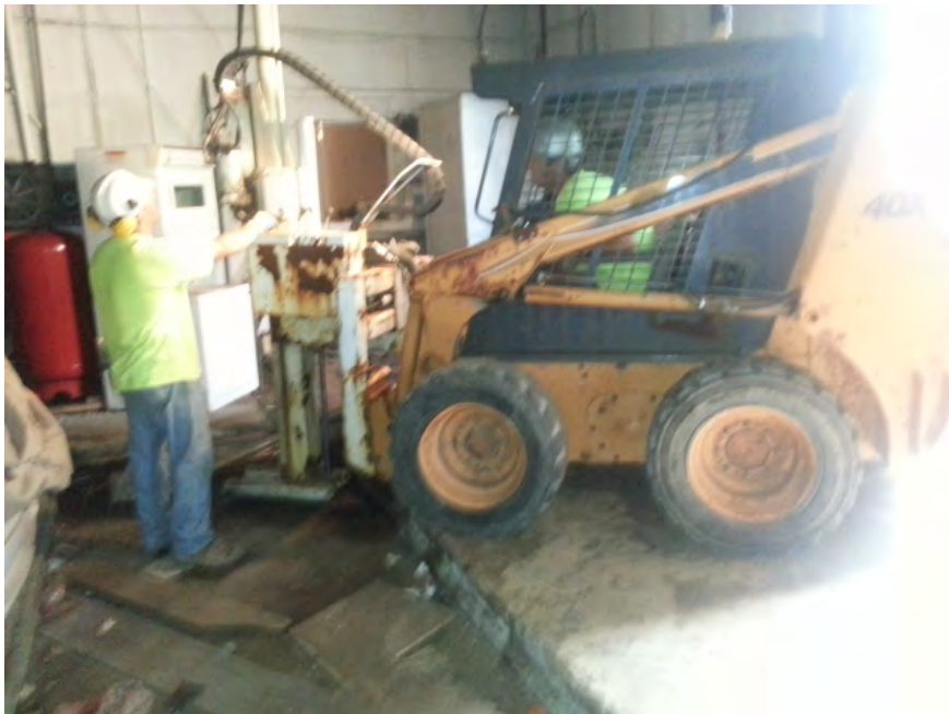
Photo 14: 08/29/13 – Hydraulic direct-push unit (geoprobe) location GS-01/CC-01.
