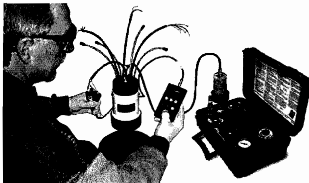
Taking pressure measurements with Model 404 Geokon Vibrating Wire Readout
