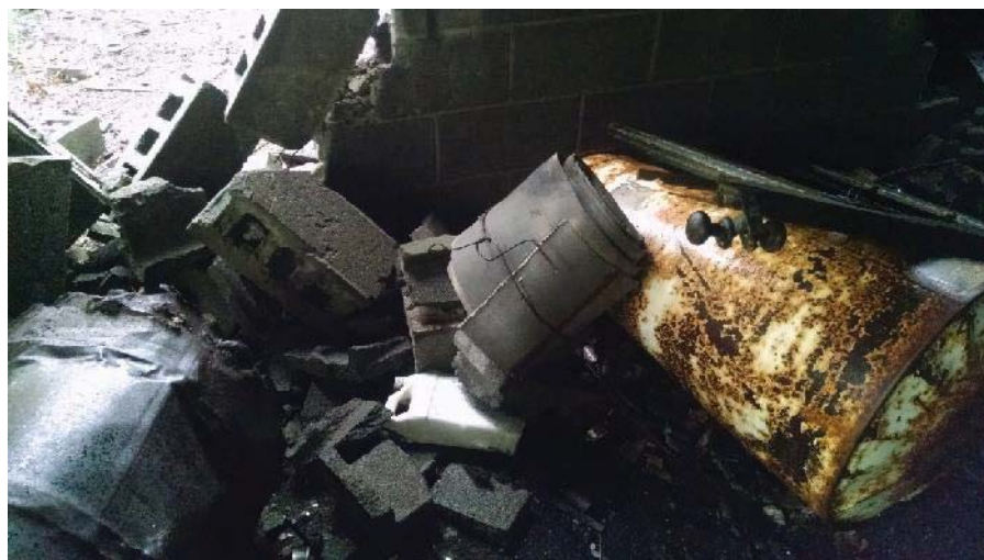
Photo 2. Homogeneous area SB1, Gray with black stripe, rolled and in pieces, woven cloth; Trace Amount of Asbestos Detected.
