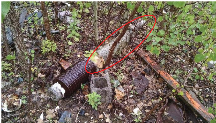
Photo 13. Homogeneous area P10-1; Brown paper wrap around electrical equipment pole; Trace Amount Asbestos Detected.
