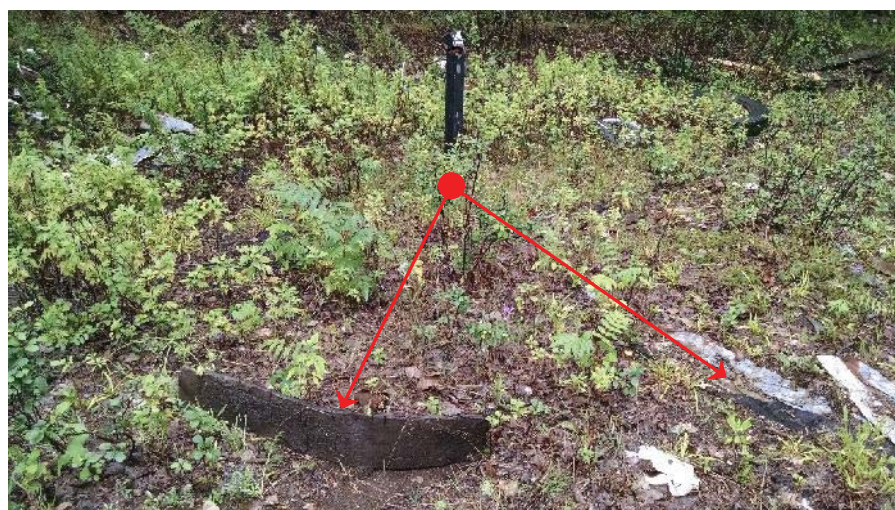
Photo 6. Homogeneous area P7-1; Black tar roofing material off of eastern corner of rubble pile 7, near monitoring well; 1.4% Chrysotile Detected.
