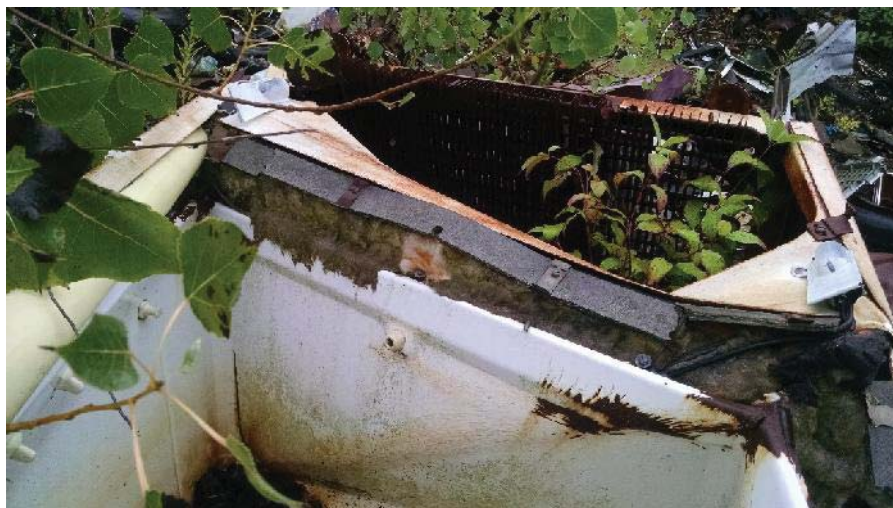
Photo 14. Homogeneous area P11-1; White wall insulation in interior of refrigerator; Trace Amount Asbestos Detected.
