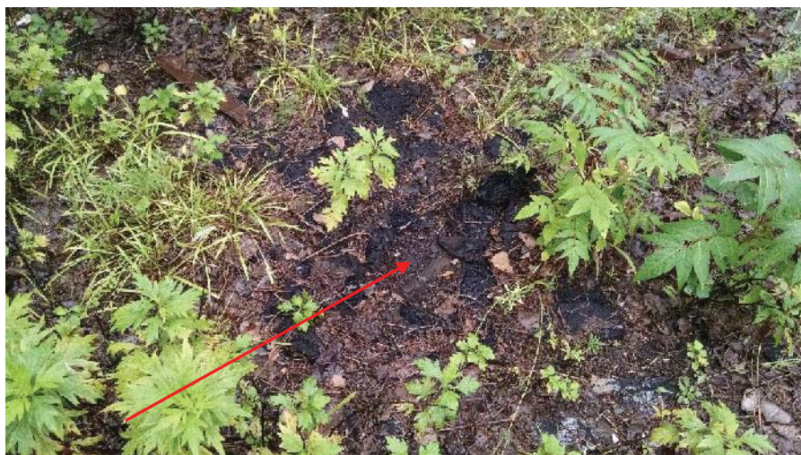
Photo 7. Homogeneous area P7-1; More black tar roofing material flattened and semi-buried in grass.
