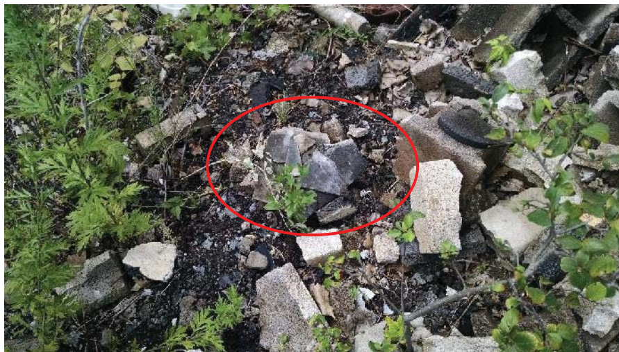
Photo 5. Homogeneous area P2-2; Light Gray (with black mastic material) transite shingle pieces; Transite shingles – 5.7% Chrysotile ; Black mastic – 15% Chrysotile .
