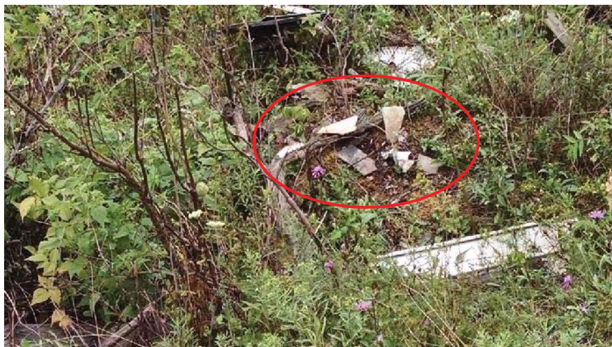
Photo 10. Homogeneous area P7-4; 9"x9" Gray floor tile with mastic; 2.5% Chrysotile- Floor Tile; 1.4% Chrysotile - Mastic Detected.
