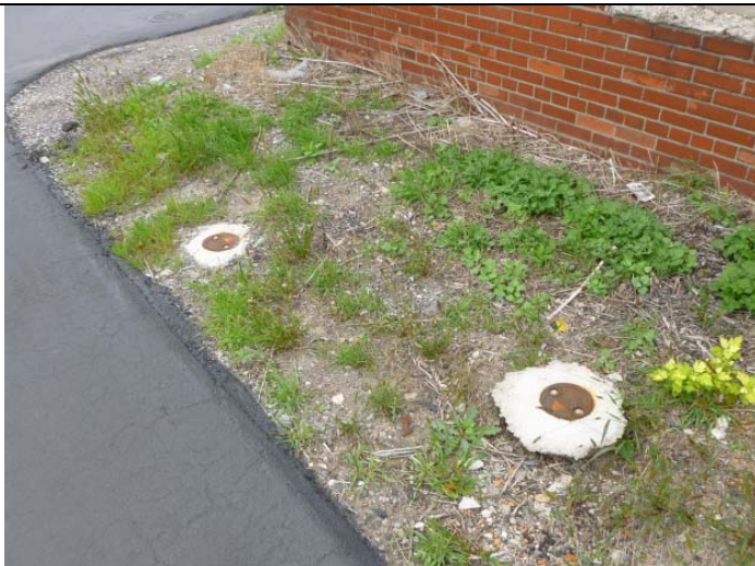
Two groundwater monitoring wells southwest of the Main Building.
