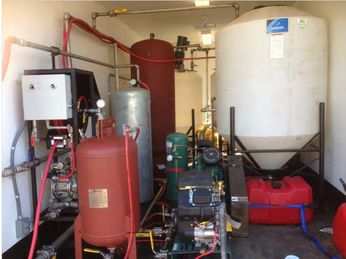
Injection Trailers Include: Multiple Liquid Feed Systems, Stainless Steel Piping, Isolated Compressed Gas Containment, Safety Shower, Eyewash Station, Onboard Generator, Chemical Resistant Construction, Mobile Office Space
