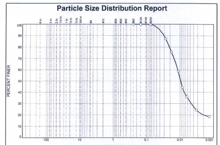
**GRAIN SIZE - mm** % Gravel % Fines % Sand % +3" Coarse Fine Coarse Medium Fine Silt Clay 0.0 0.0 0.0 0.1 68.5 0.0 0.0 31.4
