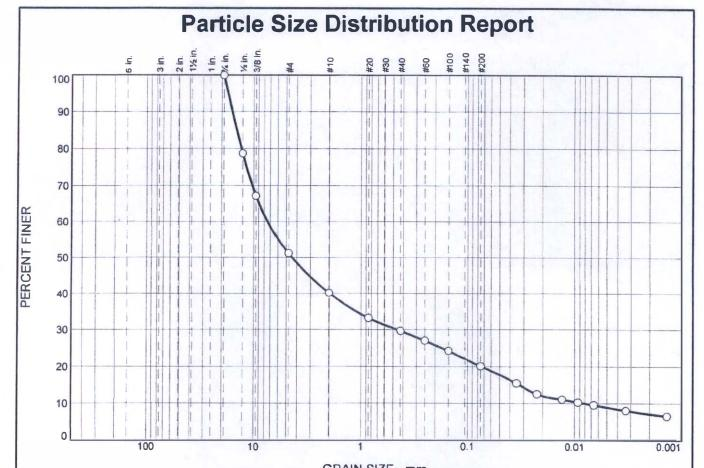
GRAIN SIZE - mm. % Gravei % Sand % Fines % +3" Coarse Fine Coarse Medium Fine Silt Clay 0.0 0.0 48.8 11.0 10.5 9.6 11.2 8.9
