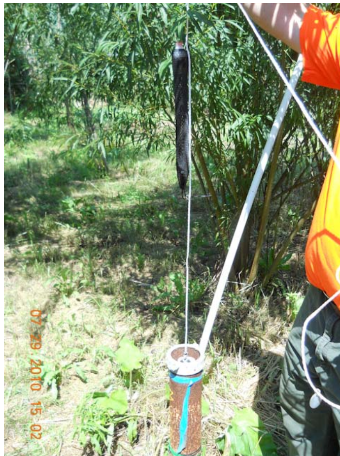
Photo #20: July 29, 2010 – PDB install at MW-9s.
