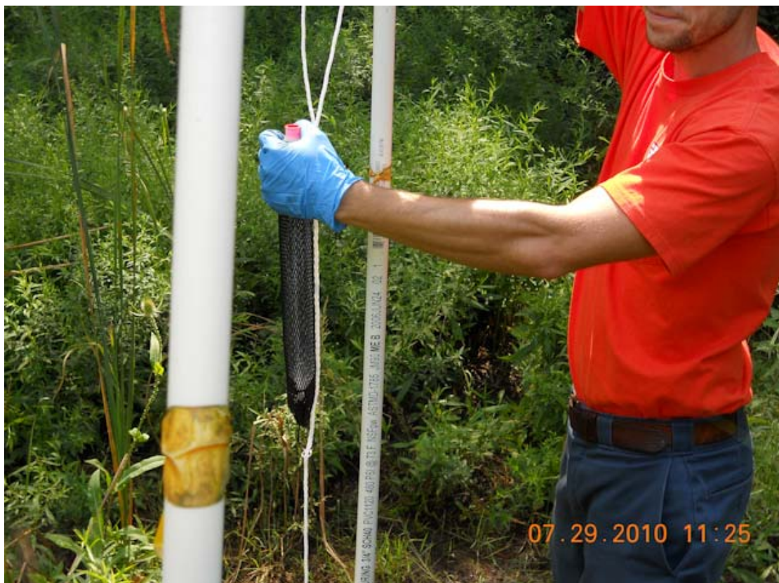
Photo #10: July 29, 2010 – PDB install at MW-4s.
