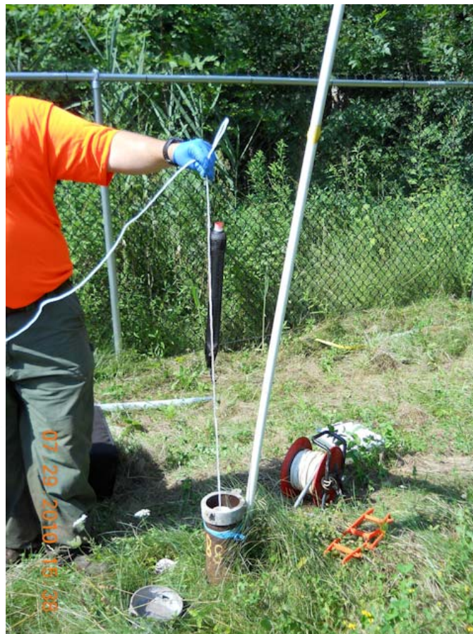
Photo #22: July 29, 2010 – PDB install at MW-8s.
