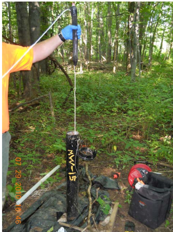
Photo #28: July 29, 2010 – PDB install at MW-15.
