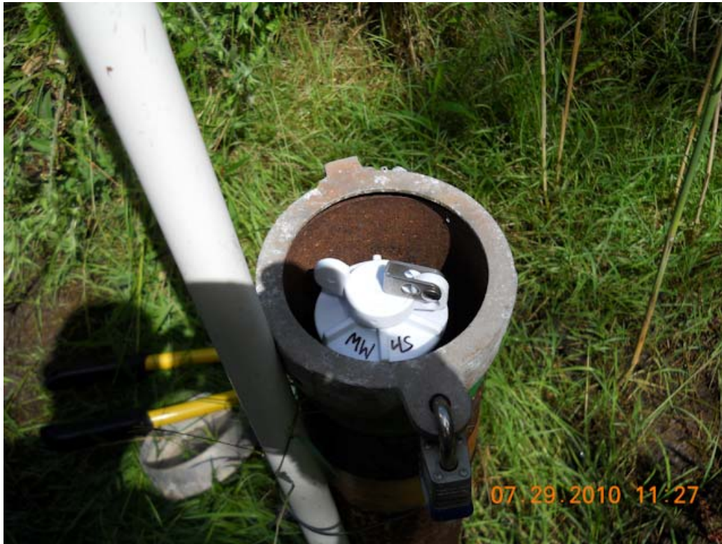
Photo #11: July 29, 2010 – PDB install at MW-4s complete.
