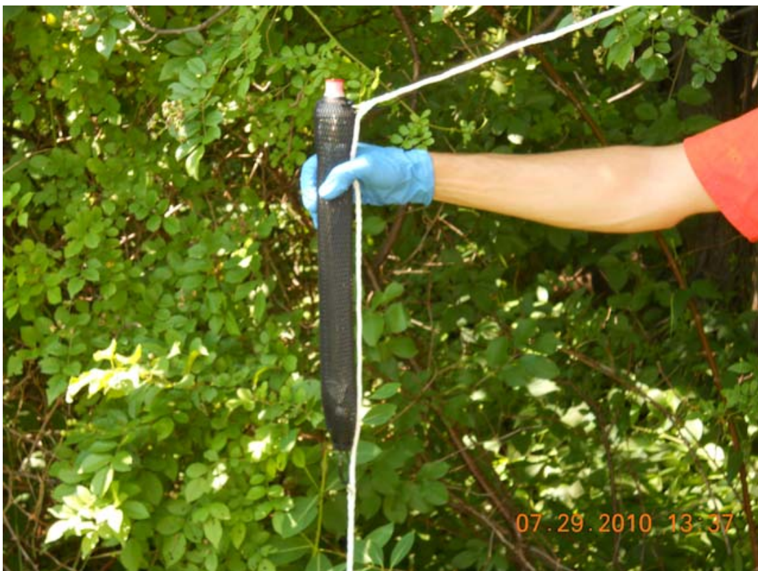
Photo #14: July 29, 2010 – PDB install at MW-6s.
