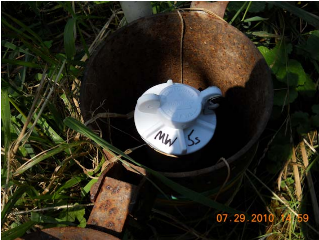
Photo #19: July 29, 2010 – PDB install complete at MW-5s.
