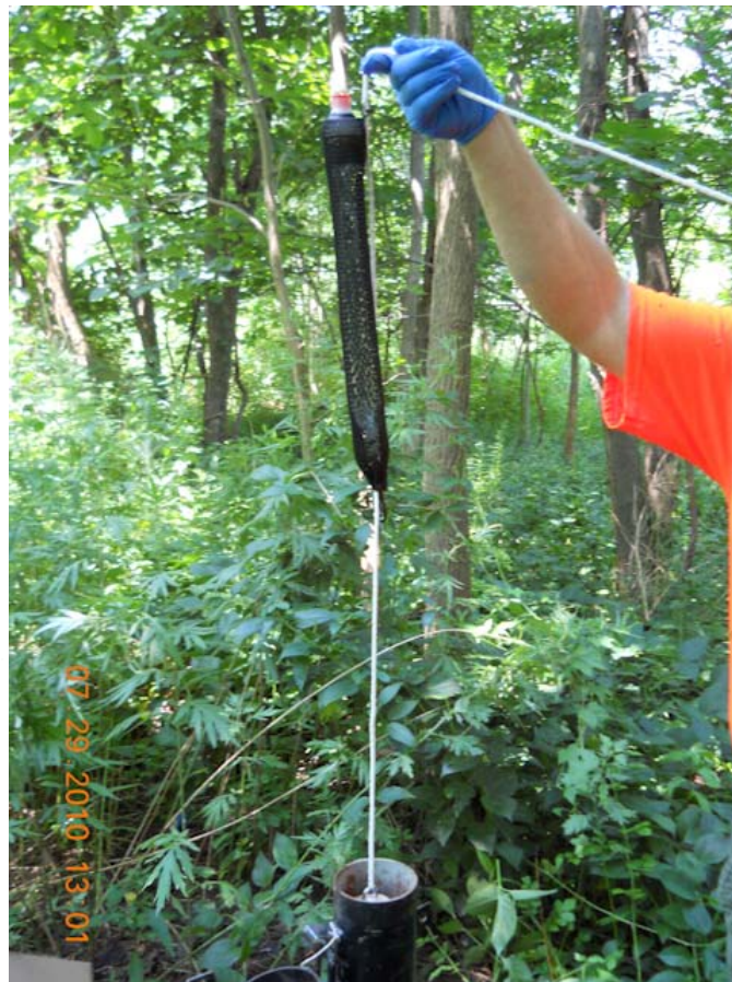
Photo #12: July 29, 2010 – PDB install at MW-17.
