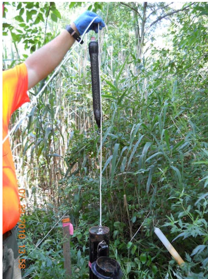
Photo #16: July 29, 2010 – PDB install at MW-16.
