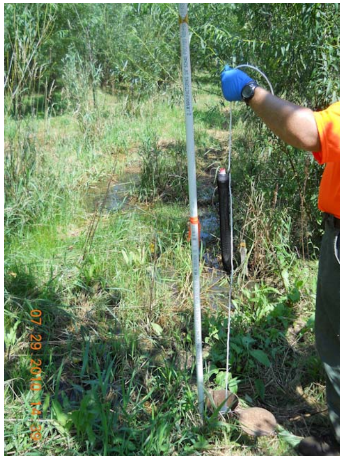
Photo #18: July 29, 2010 – PDB install at MW-5s.
