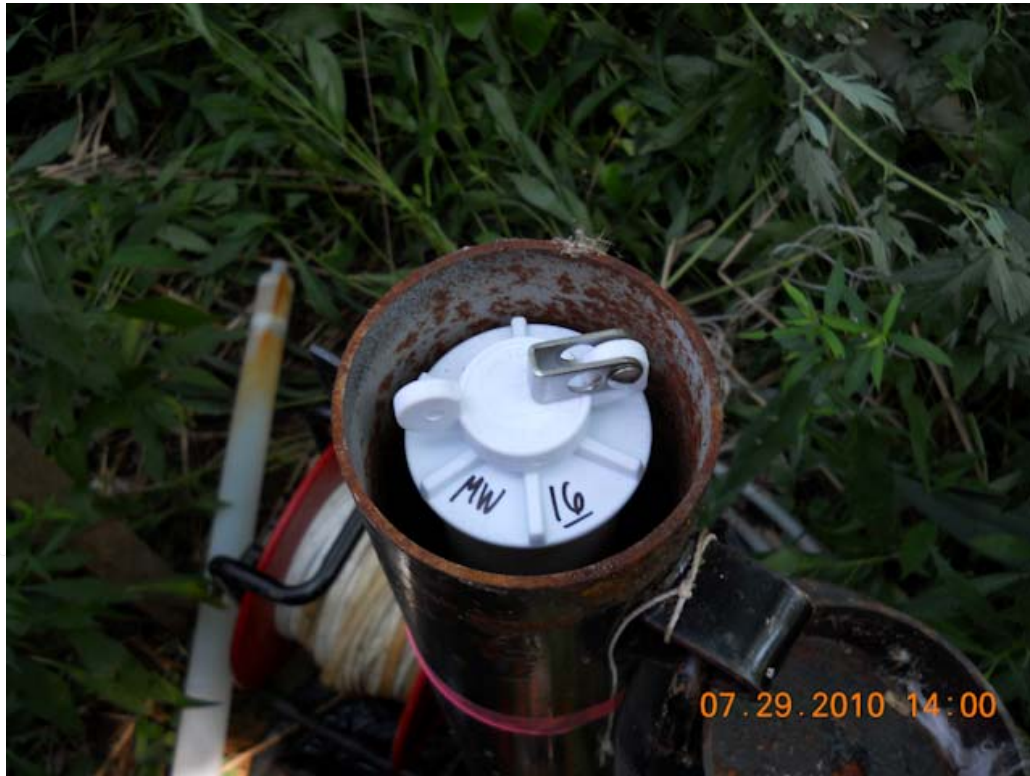
Photo #17: July 29, 2010 – PDB install complete at MW-16.
