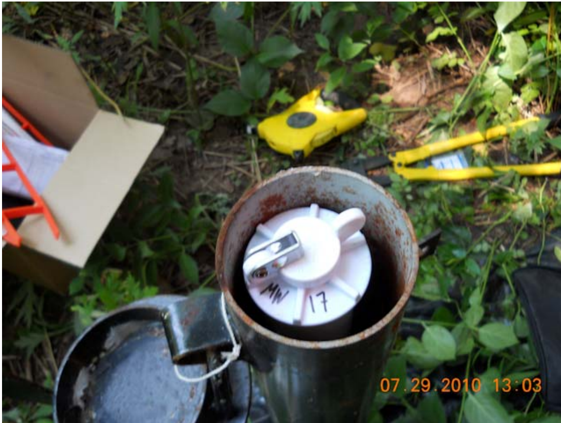
Photo #13: July 29, 2010 – PDB install at MW-17 complete.
