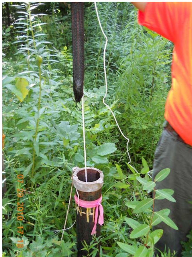
Photo #32: July 29, 2010 – PDB install at MW-14.
