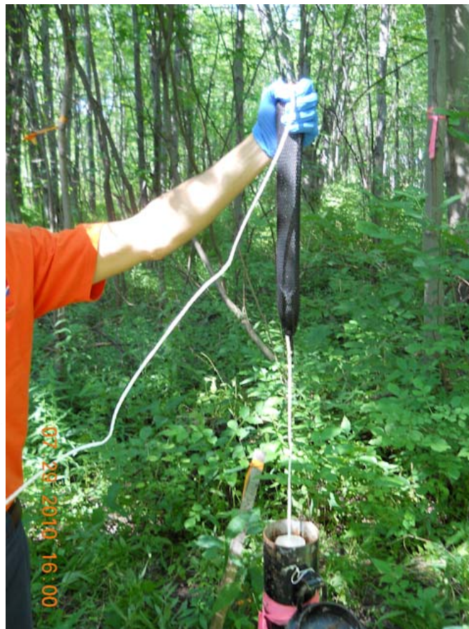
Photo #24: July 29, 2010 – PDB install at MW-18.
