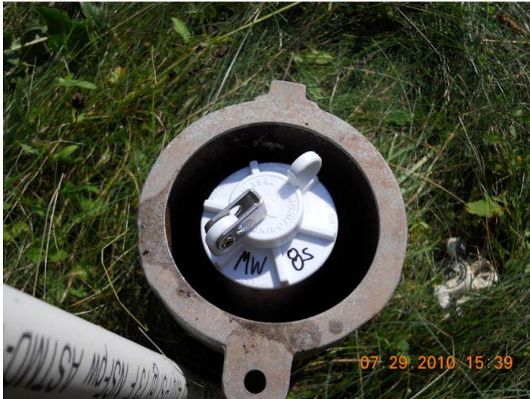
Photo #23: July 29, 2010 – PDB install complete at MW-8s.
