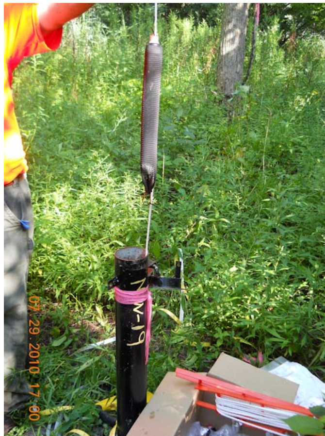
Photo #30: July 29, 2010 – PDB install at MW-19.
