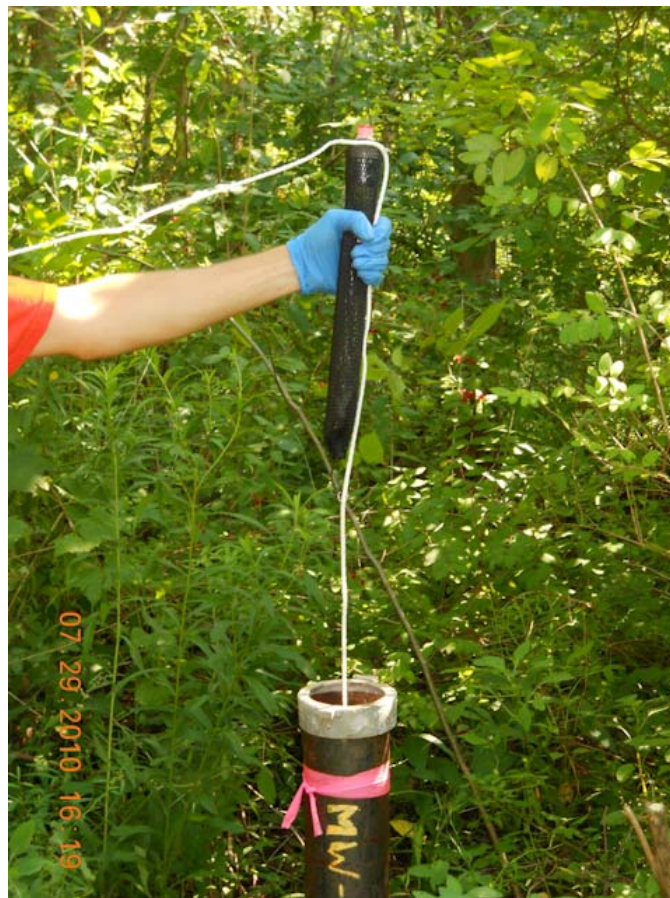
Photo #26: July 29, 2010 – PDB install at MW-13.
