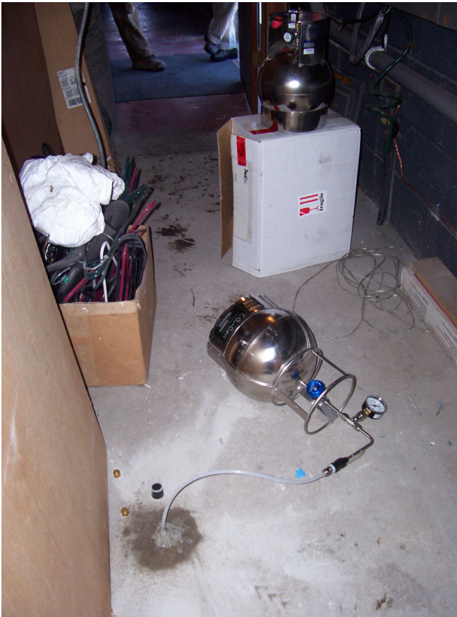
Photo #2 – Example Sub-Slab Well point Installation
