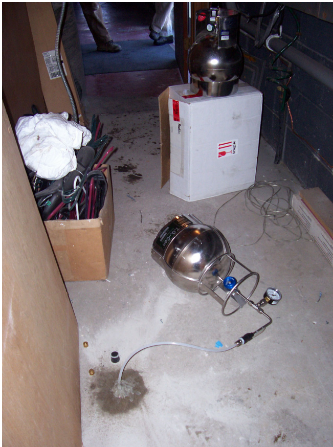
Photo #2 – Example Co-located Ambient Air /Sub-Slab Sampling Point
