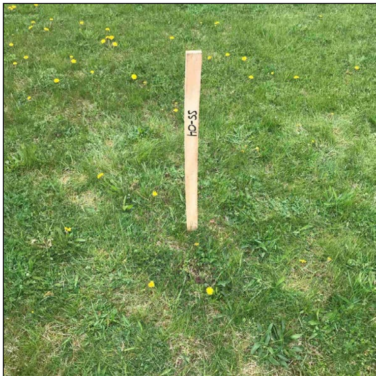
Photo Number: 12 Sample location SS04. Backfilled with soil cuttings and bentonite. --
