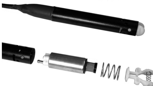
"Exploded" view of the Probe, Showing the pump, filter, spring and end cap
