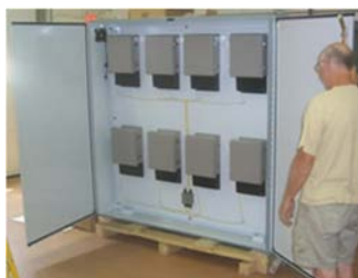
Control Boxes mounted in a NEMA enclosure
