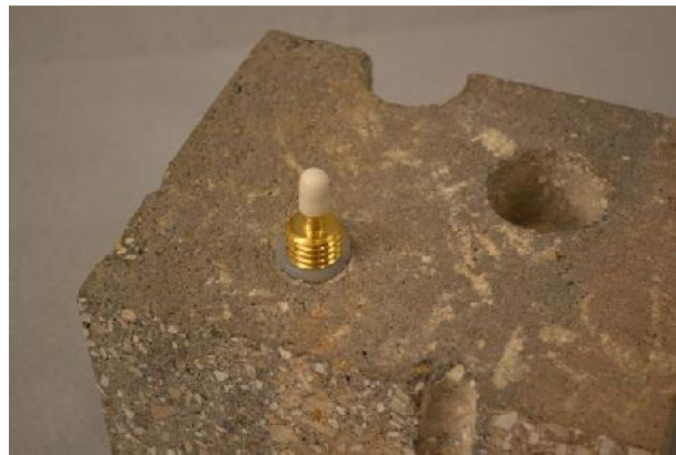
Figure 3. Installed Vapor Pin™
