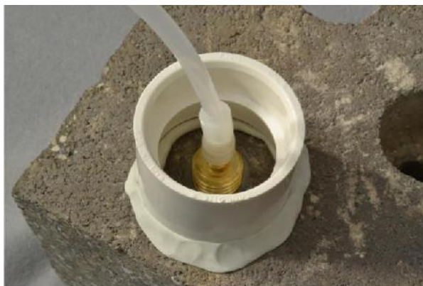
Figure 6. Water dam used for leak detection
