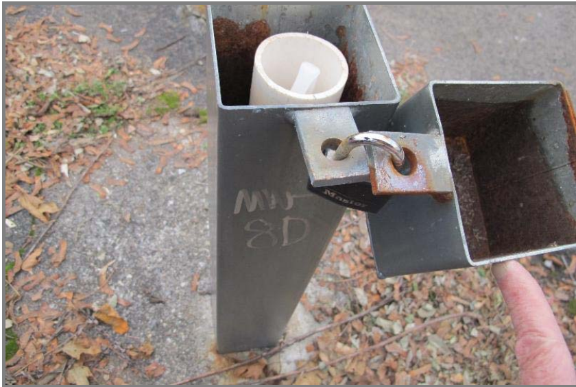
Upgradient deep well, MW-8D. Hinge is broken and cover is loose.
