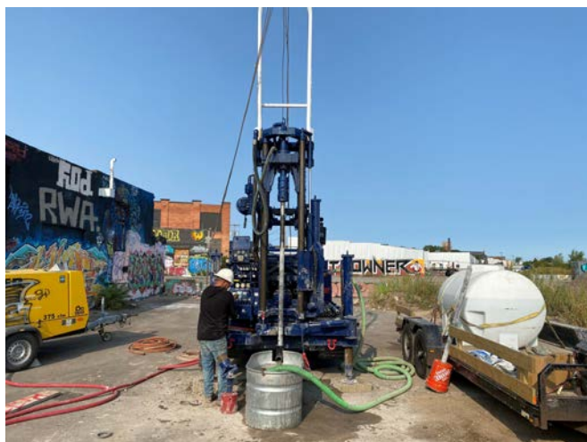
Facing west: LaBella using drilling fluid (water) and NX-core barrel to drill bedrock at IW-01. (9/16/2020)
