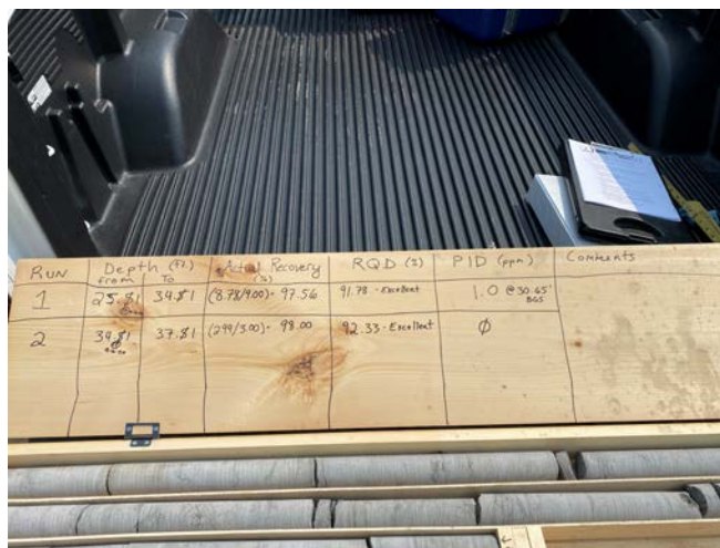
Facing east: IW-01 bedrock core and core information. (9/16/2020)
