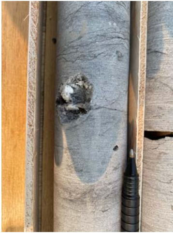
Vug-sized void space and in MW-17R NX-core with crystalline precipitate present and a pit-size void space to the left of the pen tip. (9/16/2020)
